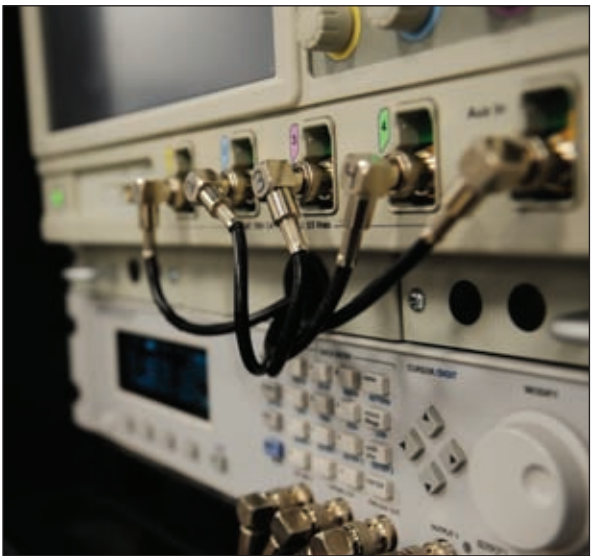
An oscilloscope, a device used to measure frequencies at Whiteman Air Force Base, Mo., Oct. 1, 2015. The avionics backshop crewmembers check the oscilloscope parameter often to ensure the integrity of the test station for line replacing unit testing.
