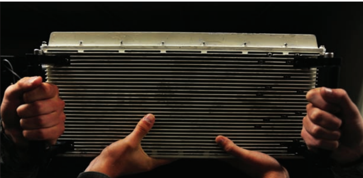
Airman 1st Class Michael Bentley and Bruno Gomes, both, 509th Maintenance Squadron avionics technicians, pick up an actuator remote terminal (ART) at Whiteman Air Force Base, Mo., Oct. 1, 2015. The ART helps stimulate B-2 spirit flight controls during operations.
