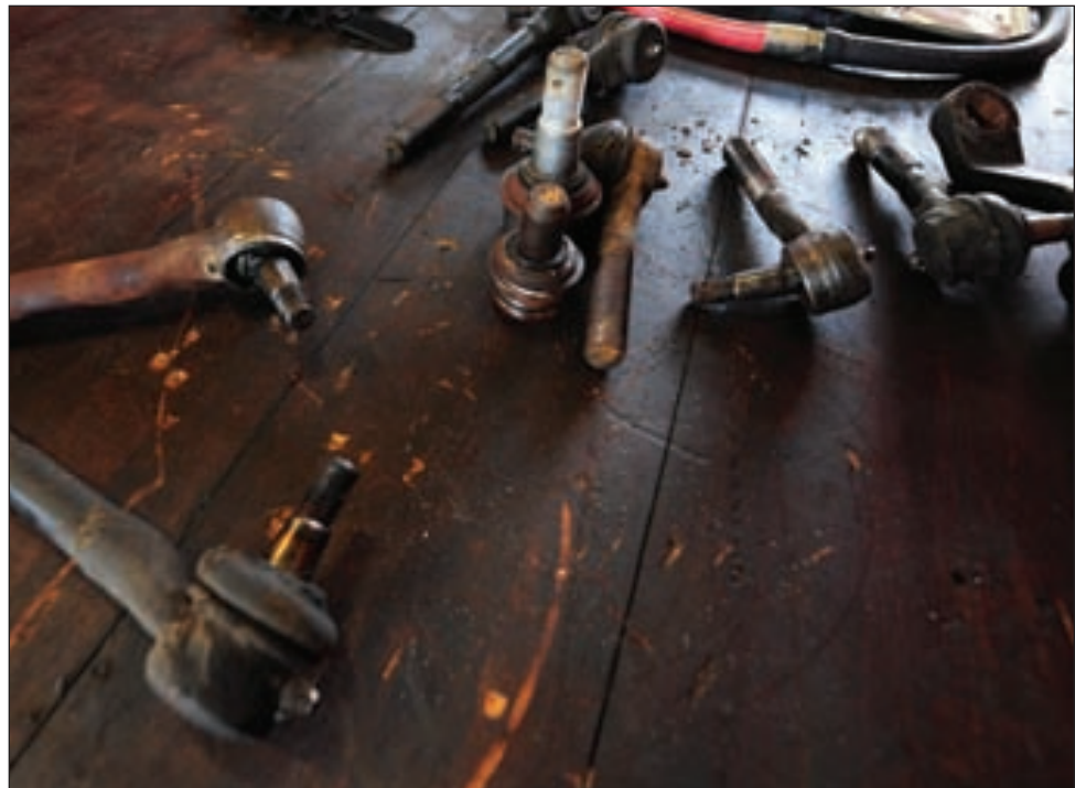
Tie rod ends lay dormant a table at Whiteman Air Force Base, Mo., Sept. 24, 2015. These parts are used to connect a vehicle's steering system to its wheels.
