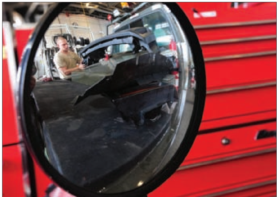
Airman 1st Class Chris Boyce, 509th Logistics Readiness Squadron vehicle maintenance journeyman, moves an upper radiator cover at Whiteman Air force Base, Mo., Sept. 24, 2015. The upper radiator cover ensures the engine fan is directing air flow toward the vehicle's engine to prevent overheating.
