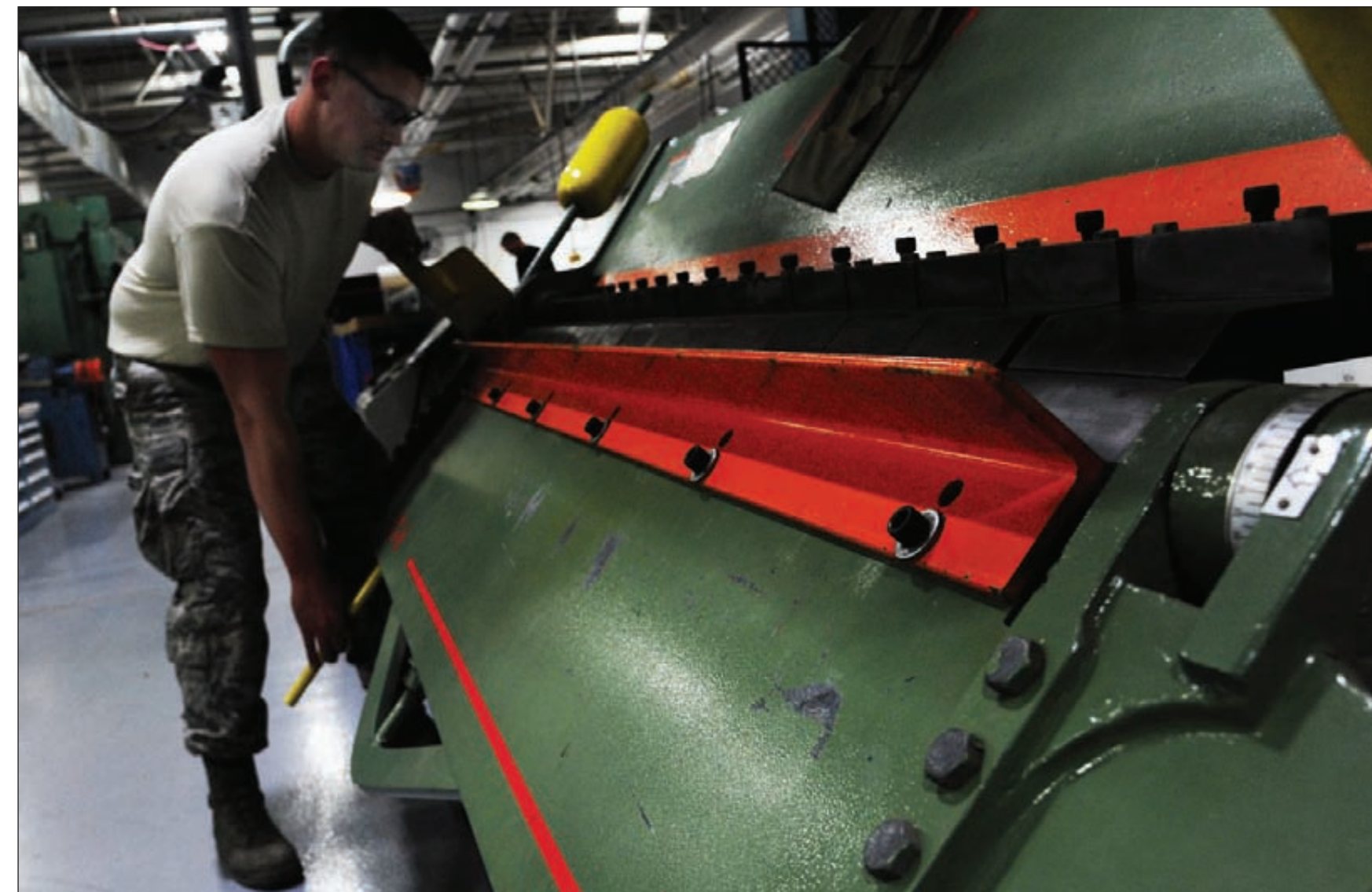
Senior Airman Cody Knott, 495th Fighter Group structural maintenance technician, bends a piece of metal at Whiteman Air Force Base, Mo., Sept. 15, 2015. Metal pieces are bent to fulfill the shape requirement for various aircraft parts.
