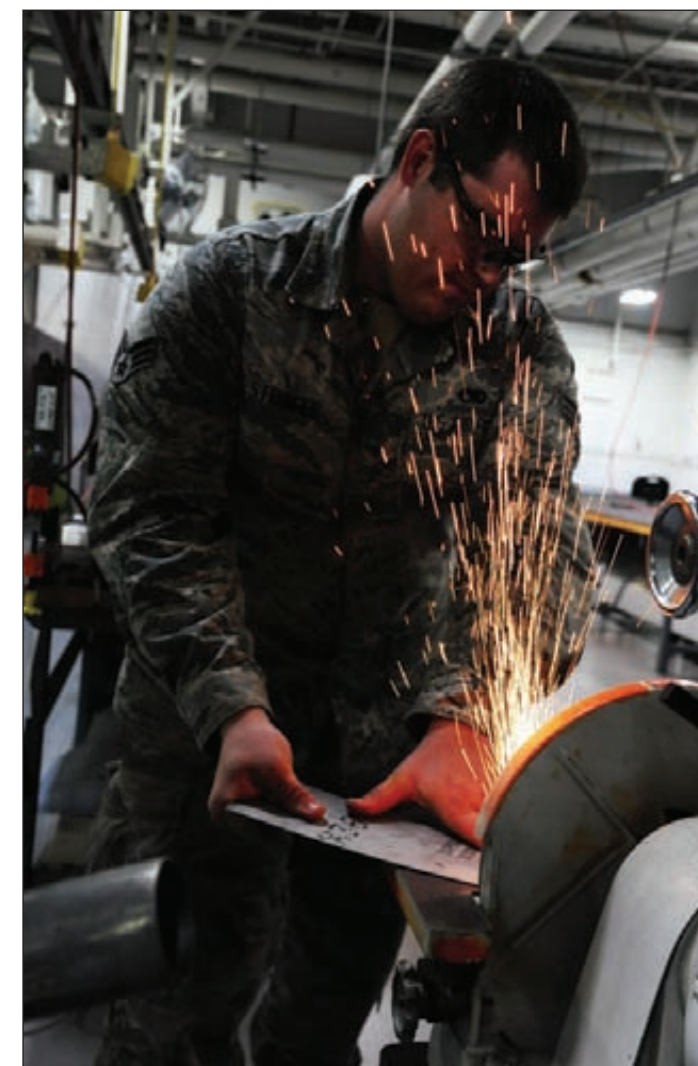
Senior Airman Spencer Stringer, 495th Fighter Group structural maintenance technician, shaves metal at Whiteman Air Force Base, Mo., Sept. 15, 2015. Parts must be shaved in order to fit properly on an aircraft.
