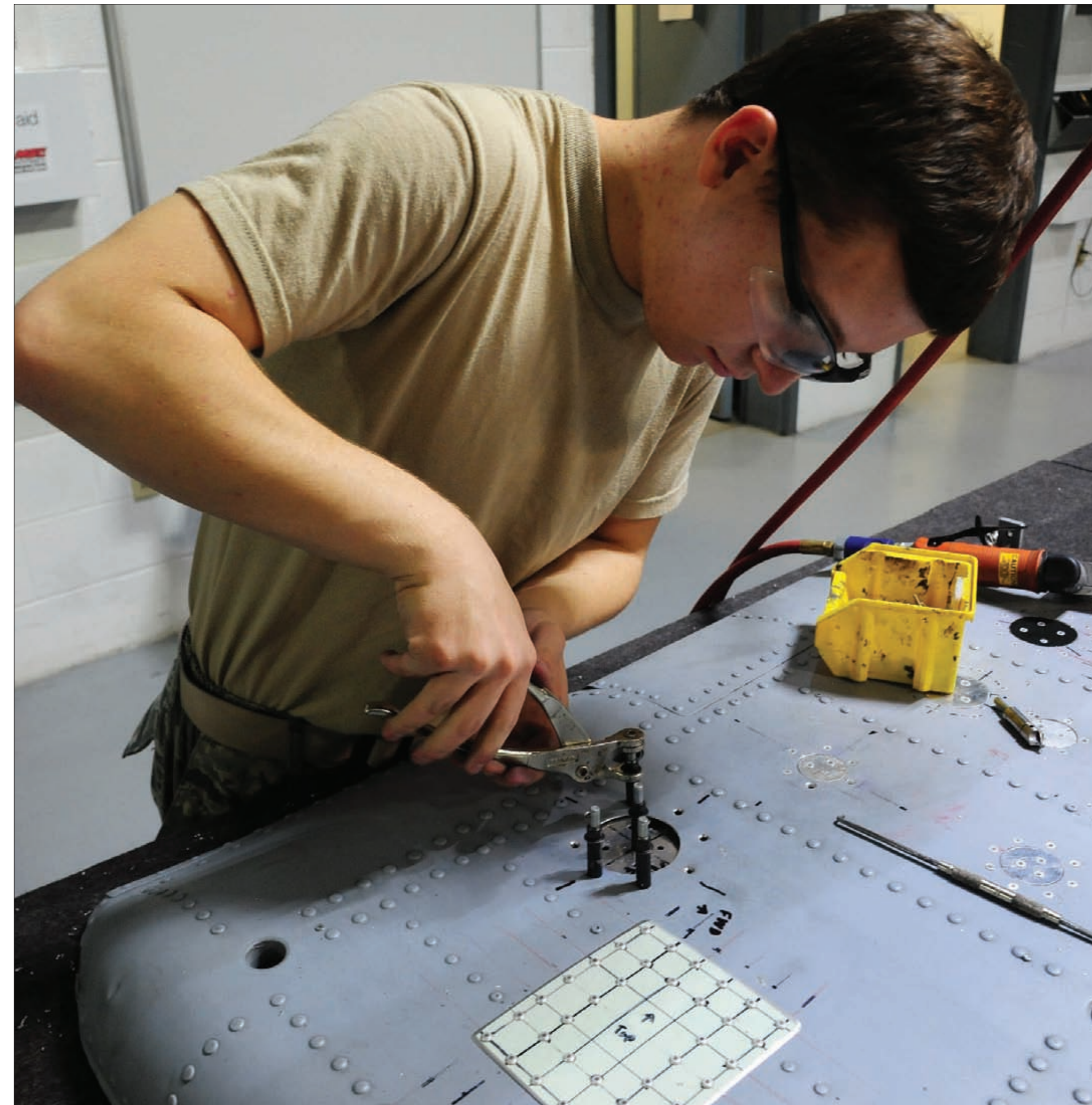
Airman 1st Class Logan Gutierrez, 509th Maintenance Squadron low observable trainee, performs a flush repair on an aircraft part at Whiteman Air Force Base, Mo., Sept. 15, 2015. Flush repairs are done to restore punctures on aircraft parts, preventing the metal from loosening or corroding.
