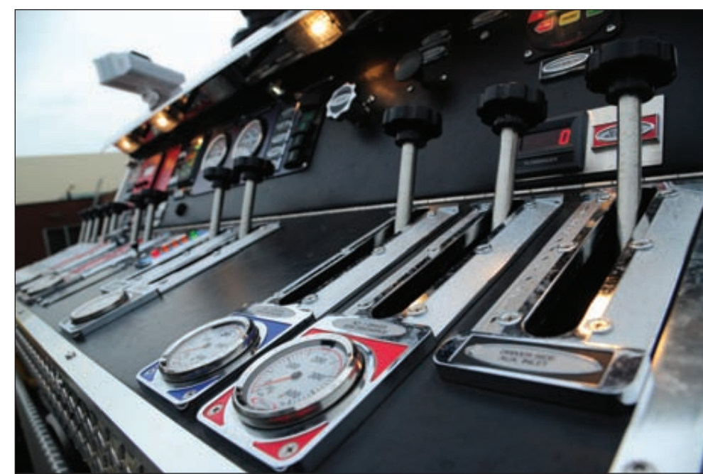
The pump panel of a fire truck remains available for emergencies at Whiteman Air Force Base, Mo., May 28, 2015. The pump panel is used to direct water flow to the appropriate hose lines.
