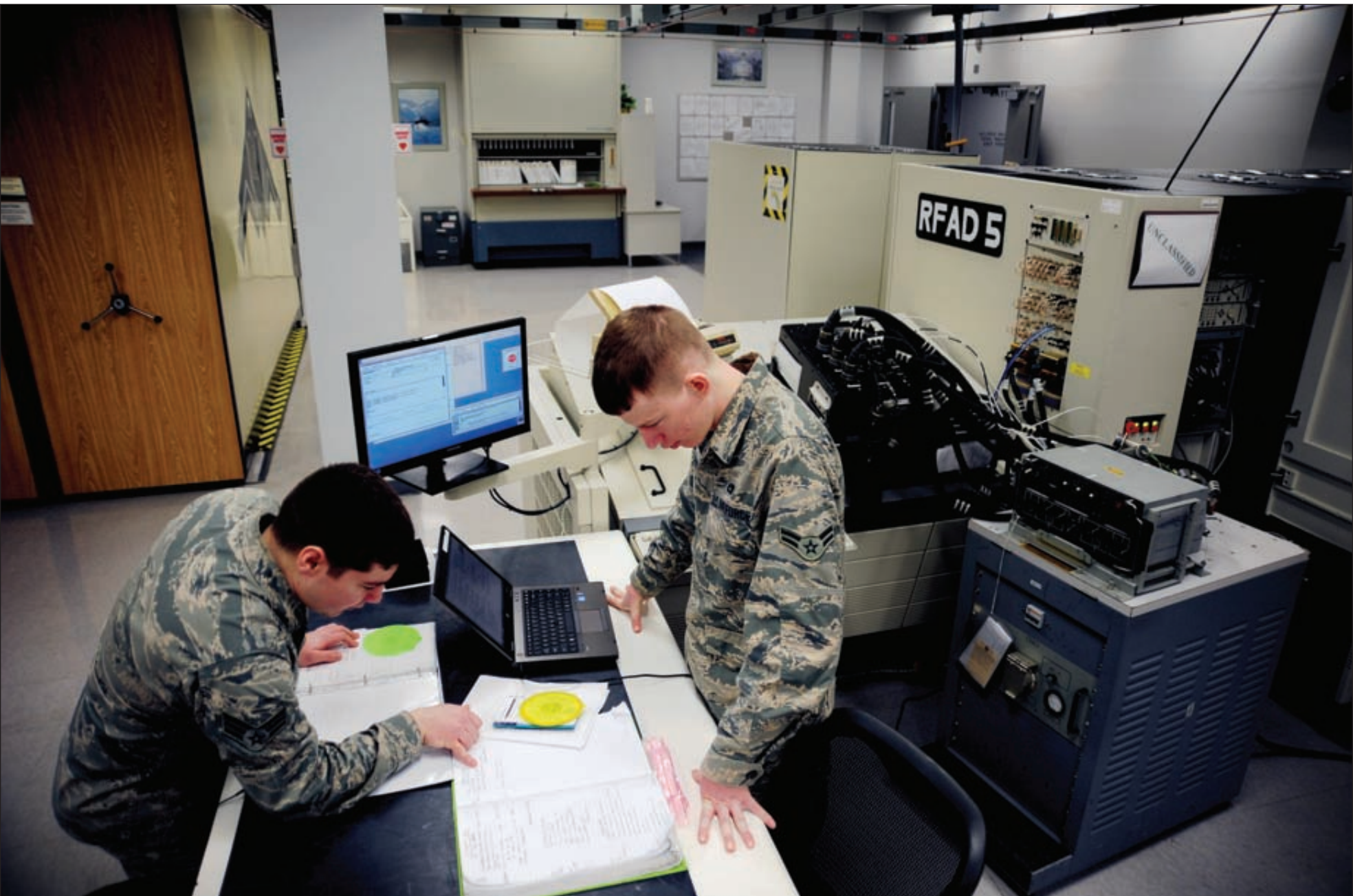
Airman 1st Class Joseph Good and Senior Airman Christopher Prescott, both 509th Maintenance Squadron avionics test station and components journeymen, use test software for a landing program at Whiteman Air Force Base, Mo., March 18, 2015. The 509th MXS avionics flight repairs more than 300 essential B-2 components a year, saving the Air Force more than $5.8 million annually.
