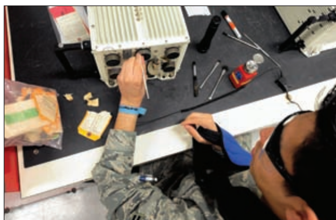
Airman 1st Class Richard Arciga, 509th Maintenance Squadron avionics test station and components journeyman, removes dust from an actuator electrical connection at Whiteman Air Force Base, Mo., March 18, 2015. Frequent removal of dust and debris helps prevent decay and rust build-up on the component.
