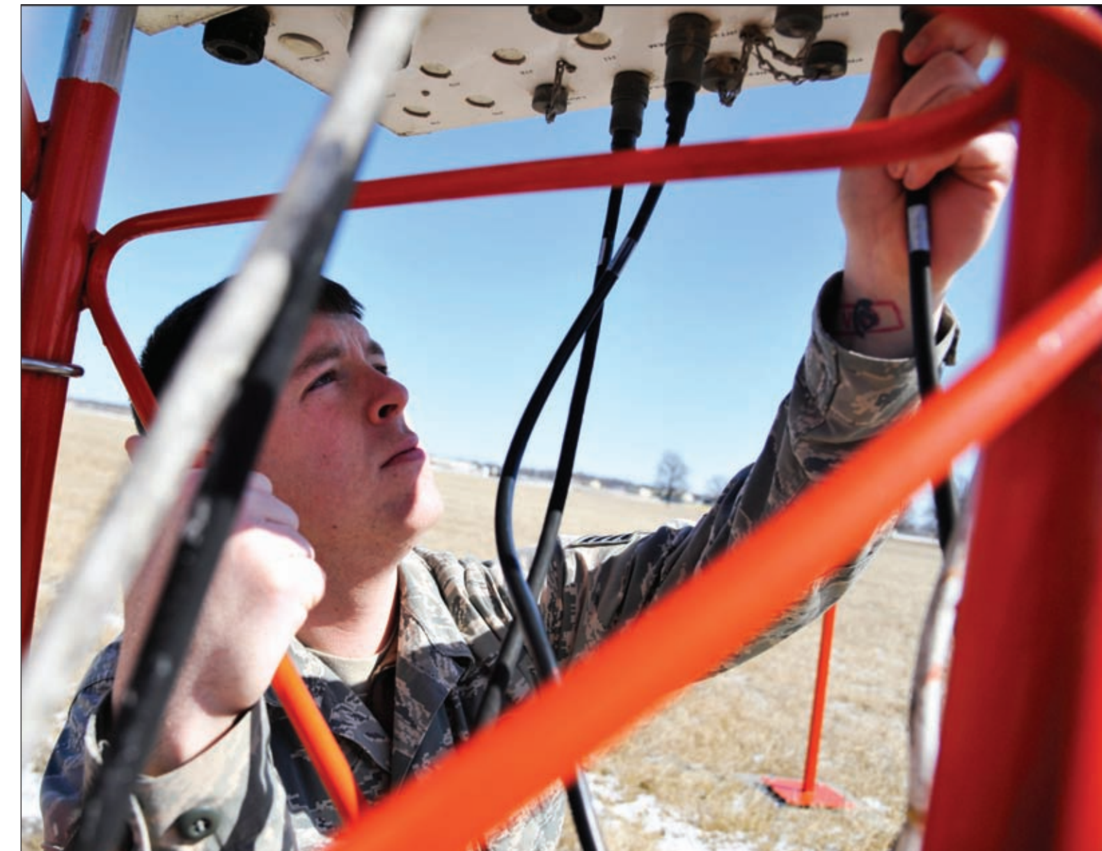
U.S. Air Force Staff Sgt. Franklyn Kapuchuck, 509th Operations Support Squadron weather forecaster, inspects an FMQ-19 weather sensor at Whiteman Air Force Base, Mo., March 5, 2015. The weather sensor measures wind speed, temperature, precipitation, visibility and cloud height.
