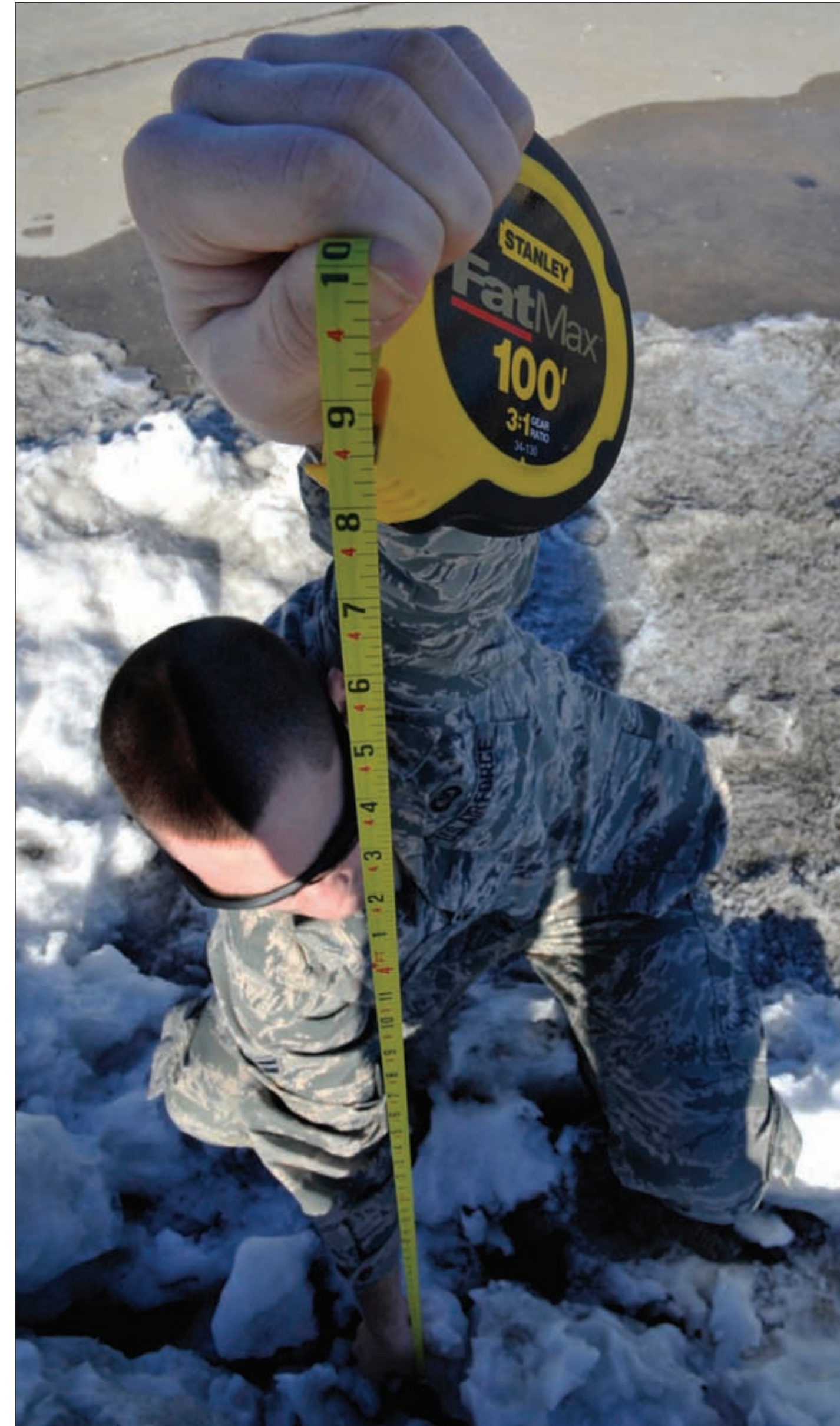
U.S. Air Force Airman 1st Class Zachary McDaniel, 509th Operations Support Squadron airfield management operations coordinator, measures snow height on the flightline at Whiteman Air Force Base, Mo., Feb. 24, 2015. Once snow height is measured, the information is reported to the Notice to Airmen (NOTAM) site for necessary precautions.
