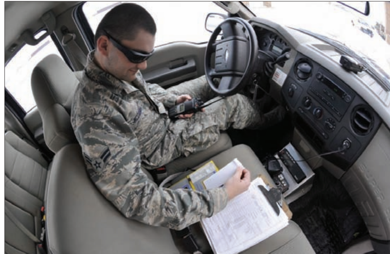
U.S. Air Force Airman 1st Class Zachary McDaniel, 509th Operations Support Squadron airfield management operations coordinator, examines decelerator results at Whiteman Air Force Base, Mo., Mar. 2, 2015. The decelerator is used to determine braking action based on how slick or dry the runways are. Once airfield management receives results, they are relayed to the pilots so they can determine the necessary braking action to use when taxiing.
