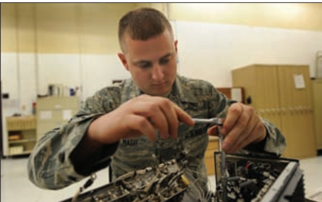
Senior Airman Colby Nash, 509th Maintenance Squadron electrical and environmental systems technician, works on a broken transformer rectifier from a B-2 Spirit, Nov. 25, 2014, at Whiteman Air Force Base, Mo. On the B-2 Spirit, systems require two different types of electricity: either alternating current or direct current. The rectifier solves this problem by taking AC power from the generators and turns it into DC for other subsystems.
