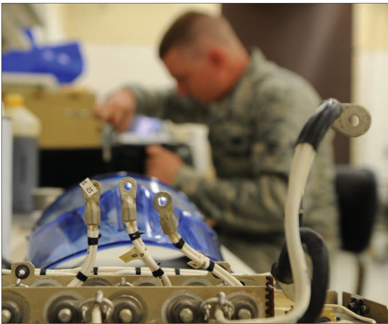
Senior Airman Colby Nash, 509th Maintenance Squadron electrical and environmental systems technician, works on a broken transformer rectifier from a B-2 Spirit, Nov. 25, 2014, at Whiteman Air Force Base, Mo. The shop was able to resolve issues of broken transformer rectifiers that could have possibly brought the shop and other maintenance personnel to a halt.
