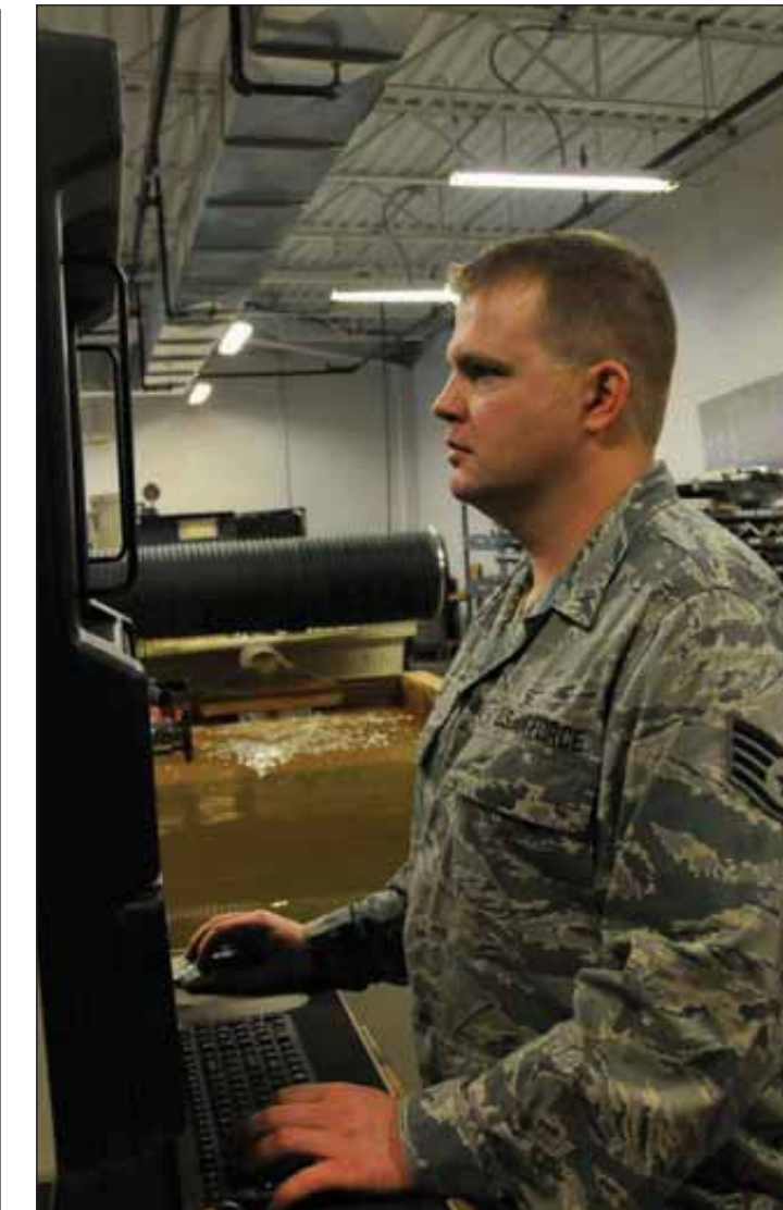
Staff Sgt. Erik Lof, 442nd Maintenance Squadron welder, programs the water jet machining center. This process cuts panels for the A-10 Thunderbolt II.
