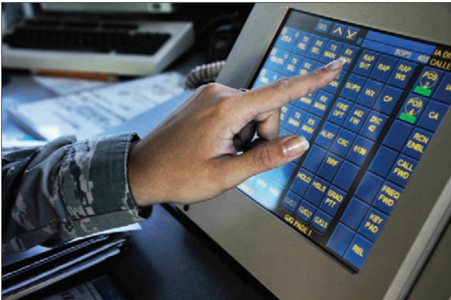
U.S. Air Force Airman 1st Class Chanel Johnson, 509th Operations Support Squadron air traffic control apprentice, operates an enhanced terminal voice switch at Whiteman Air Force Base, Mo., July 10, 2014. The enhanced terminal voice switch communicates with facilities such as base operations, and the radar, approach and control unit.
