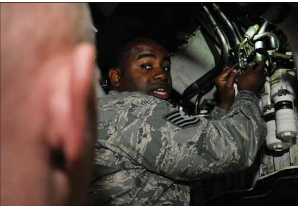
U.S. Air Force Tech. Sgt. Broderick Jones, 509th Aircraft Maintenance Squadron aircraft electrical and environmental systems craftsman, explains proper wire maintenance to Senior Airman Matthew Quick. If wire maintenance is performed poorly, it could result in damaging the aircraft.
