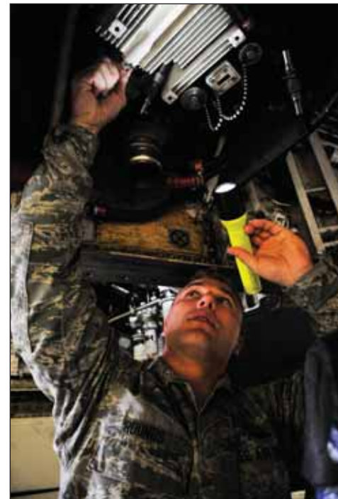
U.S. Air Force Senior Airman Dylan Rounds, 509th Aircraft Maintenance Squadron aerospace systems propulsion journeyman, inspects an auxiliary power unit. The chip detector must be inspected ensure there is no contamination inside the oil.
