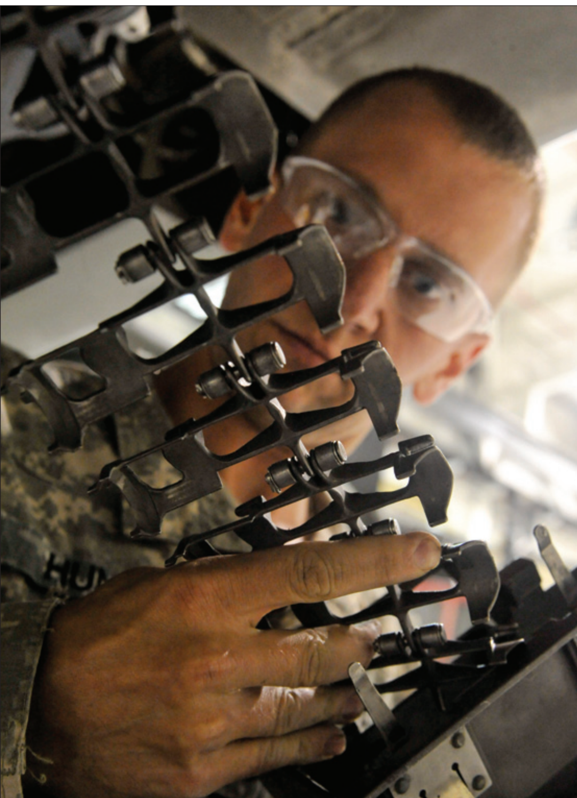
Staff Sgt. Matthew Hunt, 1-135th Attack Reconnaissance Battalion Delta Company avionics electronic armament specialist, removes a 30 mm mounted gun from an AH-64 Apache at Whiteman Air Force Base, Mo., May 14, 2014. This is a part of the annual inspections, which consists of lubing and cleaning the gun to extend its "life."
