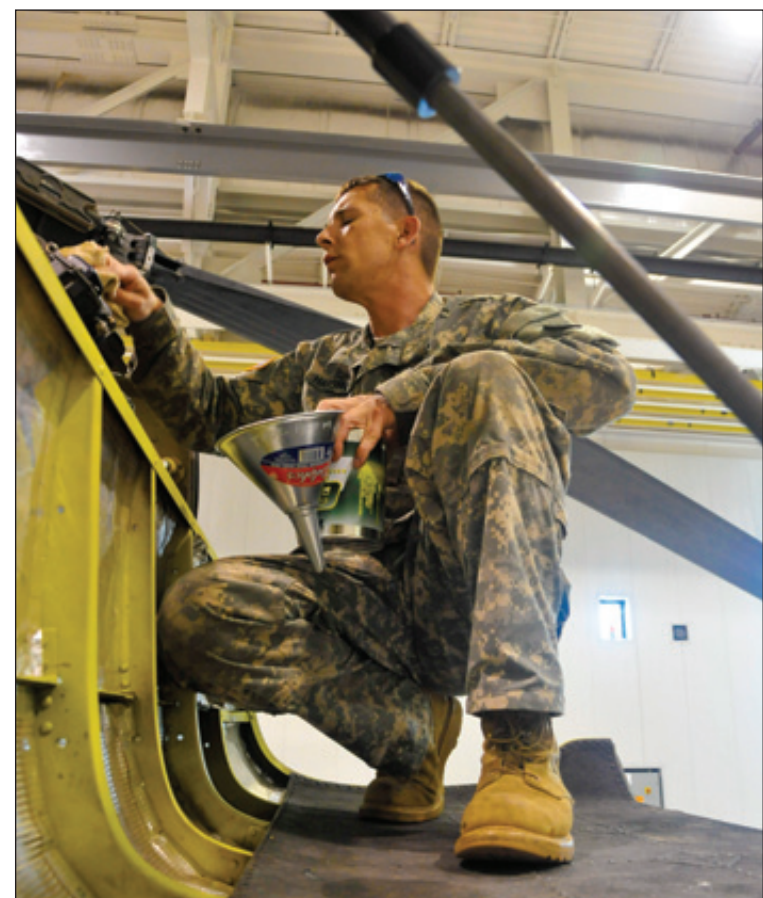
Sgt. Jeremy Harshner, 1-135th Attack Reconnaissance Battalion Delta Company avionics electronic armament specialist, fills an AH-64 Apache engine with oil at Whiteman Air Force Base, Mo., May 14, 2014. This is done to ensure the aircraft is prepared for flight.
