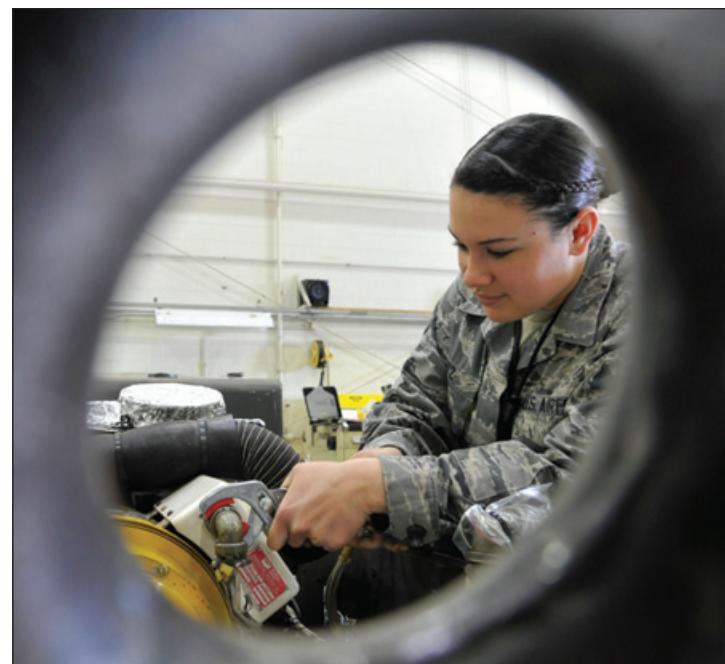
LEFT: Airman 1st Class Lance Lockett, 509th Maintenance Squadron aerospace ground equipment apprentice, removes a hydraulic line from a 30-ton jack. This task is done in preparation for a new paint job, which helps prevent corrosion from occurring on jack. RIGHT: Airman 1st Class Laura Reitz, 509th Maintenance Squadron aerospace ground equipment journeyman, loosens a cannon plug on a negative 60 gas turbine compressor. The compressor is used to supply power and compressed air to the aircraft.
