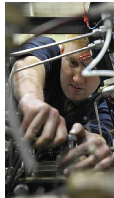
Staff Sgt. Glenn Trent, 509th Maintenance Squadron aerospace ground equipment craftsman, tightens a bolt on a self-generating nitrogen servicing cart. The nitrogen servicing carts are used to supply nitrogen to the B-2 Spirit's tires.
