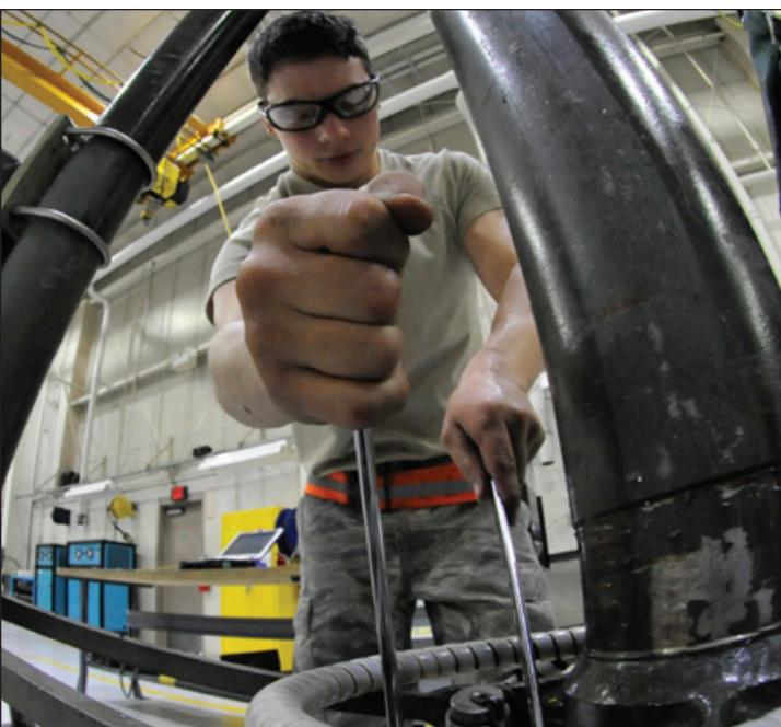
LEFT: Airman 1st Class Lance Lockett, 509th Maintenance Squadron aerospace ground equipment apprentice, removes a hydraulic line from a 30-ton jack. This task is done in preparation for a new paint job, which helps prevent corrosion from occurring on jack. RIGHT: Airman 1st Class Laura Reitz, 509th Maintenance Squadron aerospace ground equipment journeyman, loosens a cannon plug on a negative 60 gas turbine compressor. The compressor is used to supply power and compressed air to the aircraft.
