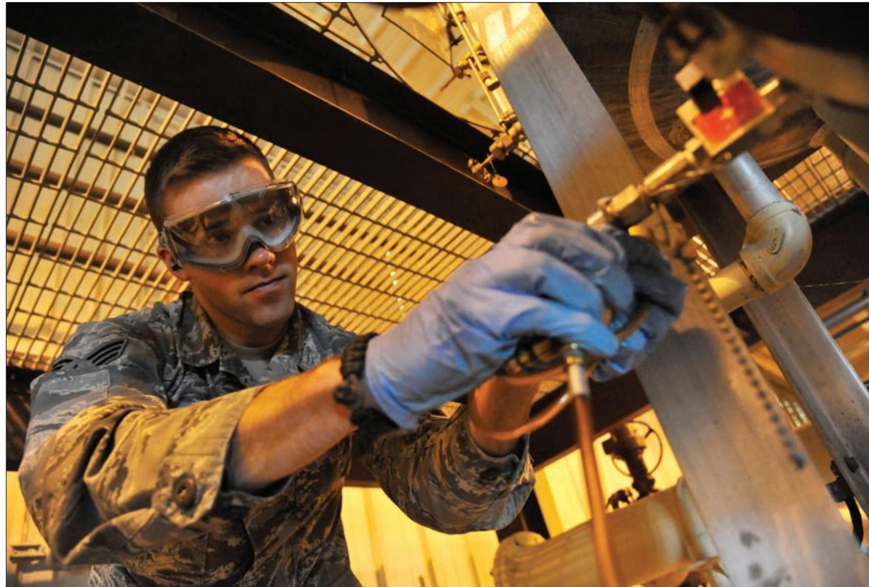
Senior Airman Dustin Cournoyer, 509th Logistics Readiness Squadron fuels laboratory technician, removes a single weight from a sampler at Whiteman Air Force Base, Mo. April 1, 2014. This portion of the weekly inspection ensures there is no sediment within the fuel.
