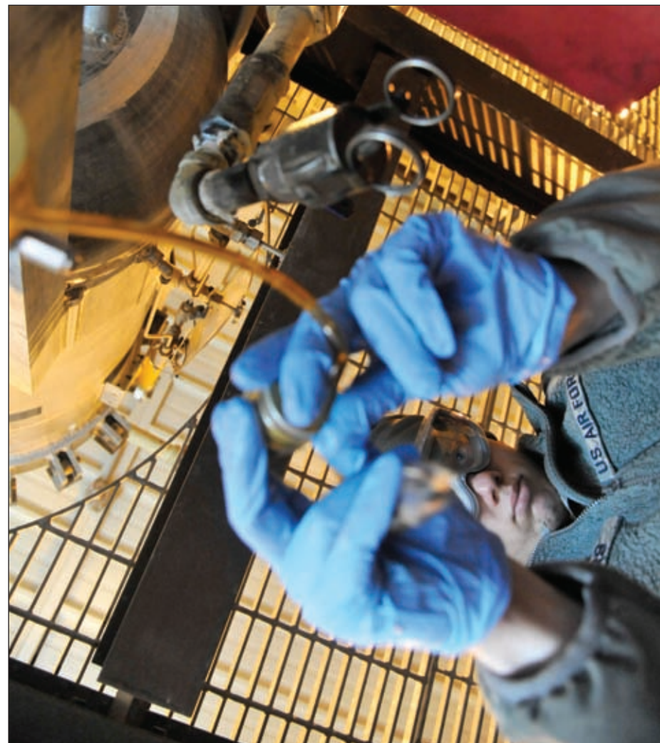
Staff Sgt. Preston Sowers, 509th Logistics Readiness Squadron NCO in charge of fuels laboratory, removes a single weight from a sampler. Removing the single weight ensures there is no sediment within the fuel. Sediment in the fuel can cause the aircraft to malfunction.
