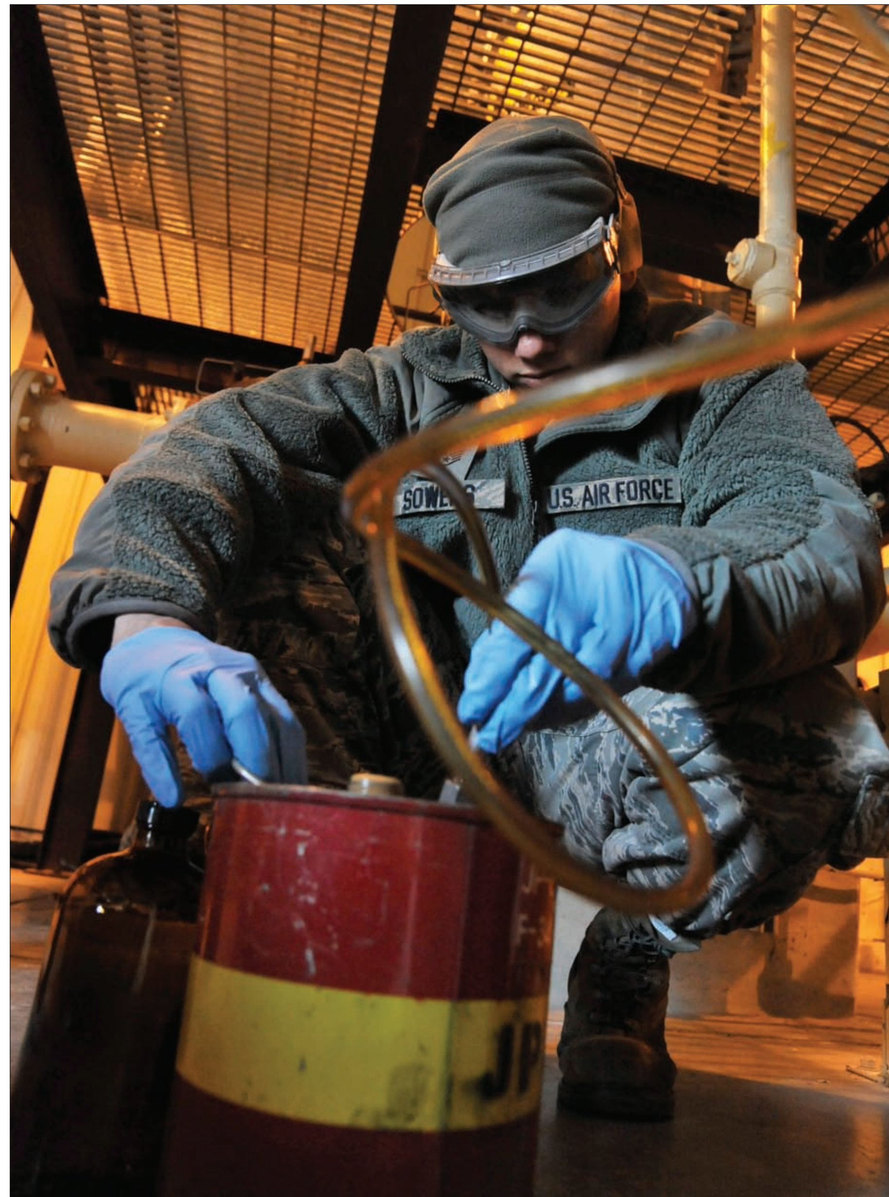
Staff Sgt. Preston Sowers, 509th Logistics Readiness Squadron NCO in charge of fuels laboratory, pulls a sample from fuel filter separators. A weekly sample from fuel separators is taken to ensure it contains no water or sediments.
