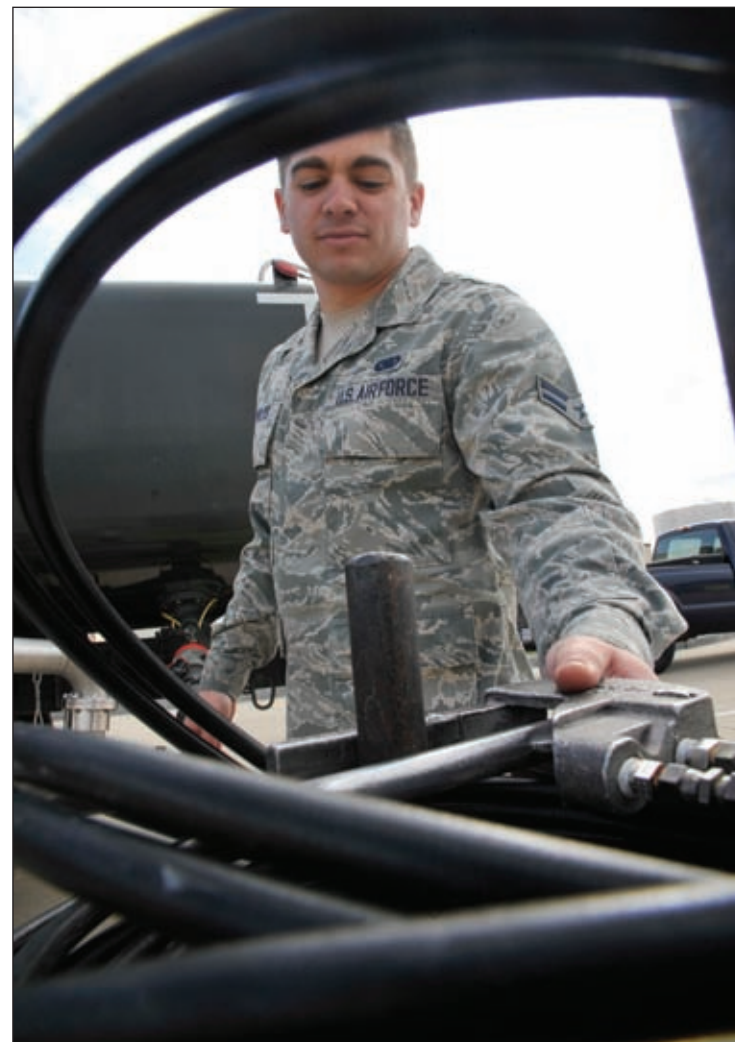
Airman 1st Class Joshua Reynolds, 509th Logistics Readiness Squadron fuels distribution technician, puts down a "dead man" control. The "dead man" control activates the fuels stand to fuel R11 trucks.
