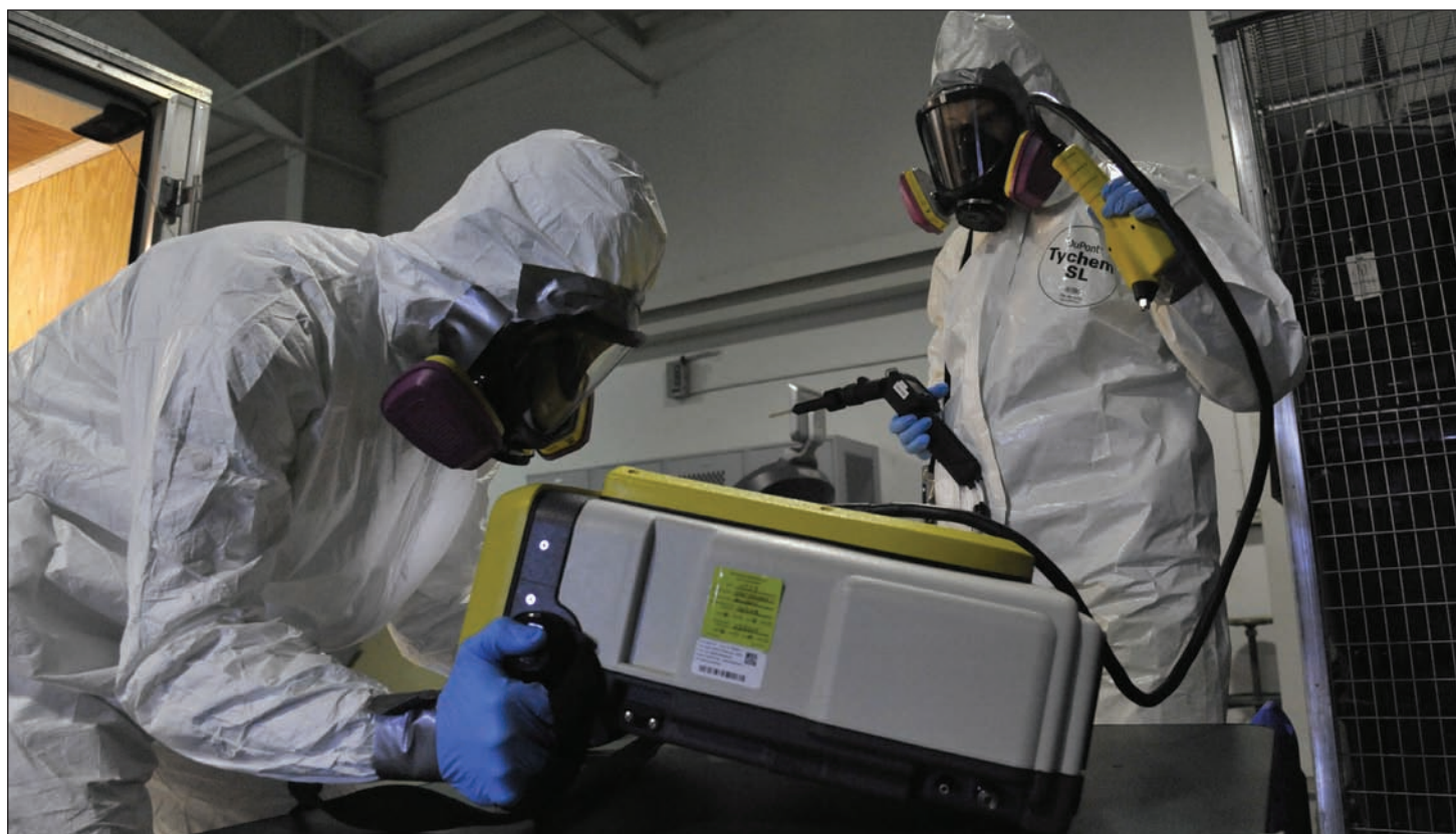
Staff Sgt. Tyler Haugland, 509th Medical Operations Squadron bioenvironmental readiness and radiation program manager, left, and Tech. Sgt. Annemieke LeBorgne, 509th Medical Operations Squadron NCO in charge of Occupational Health, prepares the HAPSITE. The HAPSITE is used to identify and quantify potential unknowns.
