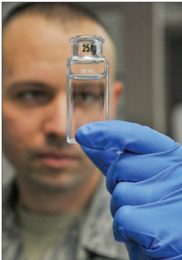
U.S. Air Force photo/Airman 1st Class Keenan Berry U.S. Air Force Senior Airman Brandon Lynn, 509th Civil Engineer Squadron water and fuels maintenance journeyman, performs a chlorine residual test at Whiteman Air Force Base, Mo., March 3, 2014. This procedure is done to ensure chlorine residual is within the required ranges for achievable disinfection.
