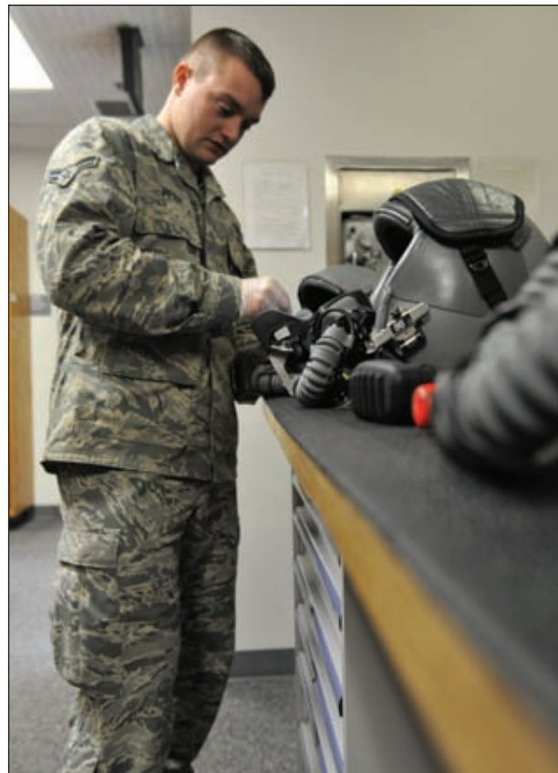
Airman 1st Class Brandon Perry, 509th Operations Support Squadron aircrew flight equipment technician, sanitizes an MBU-20/P soft shell mask. AFE technicians clean the insides of the masks to ensure there are no contaminants, debris or germs in the mask.
