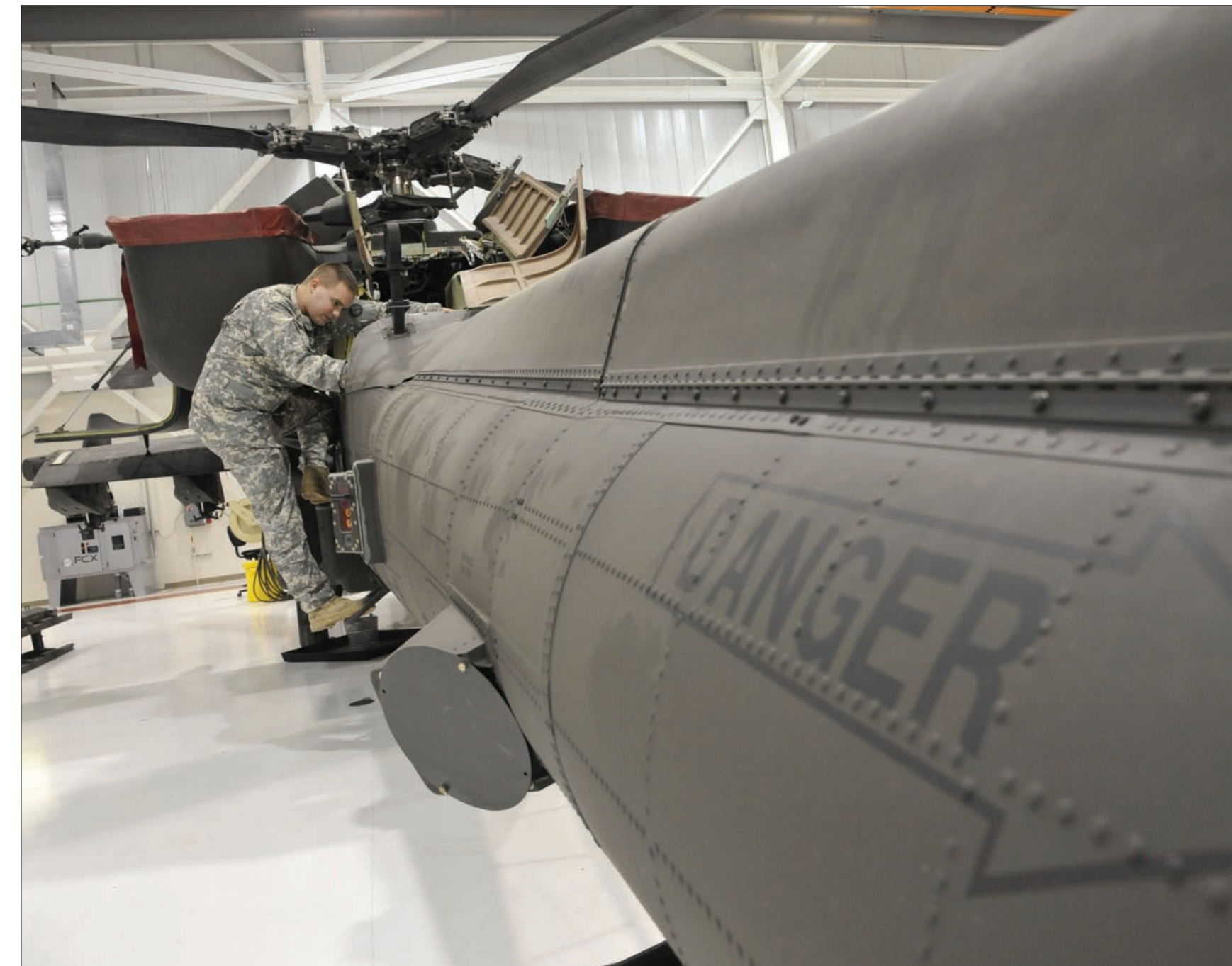
U.S. Army Spc. Todd Gann, 1-135th Attack/Reconnaissance Battalion aircraft maintainer, checks bearings for axial movement within the tail of an AH-64 Apache at Whiteman Air Force Base, Mo., Jan. 9, 2014. This inspection ensures the aircraft will maintain its stability while in flight.
