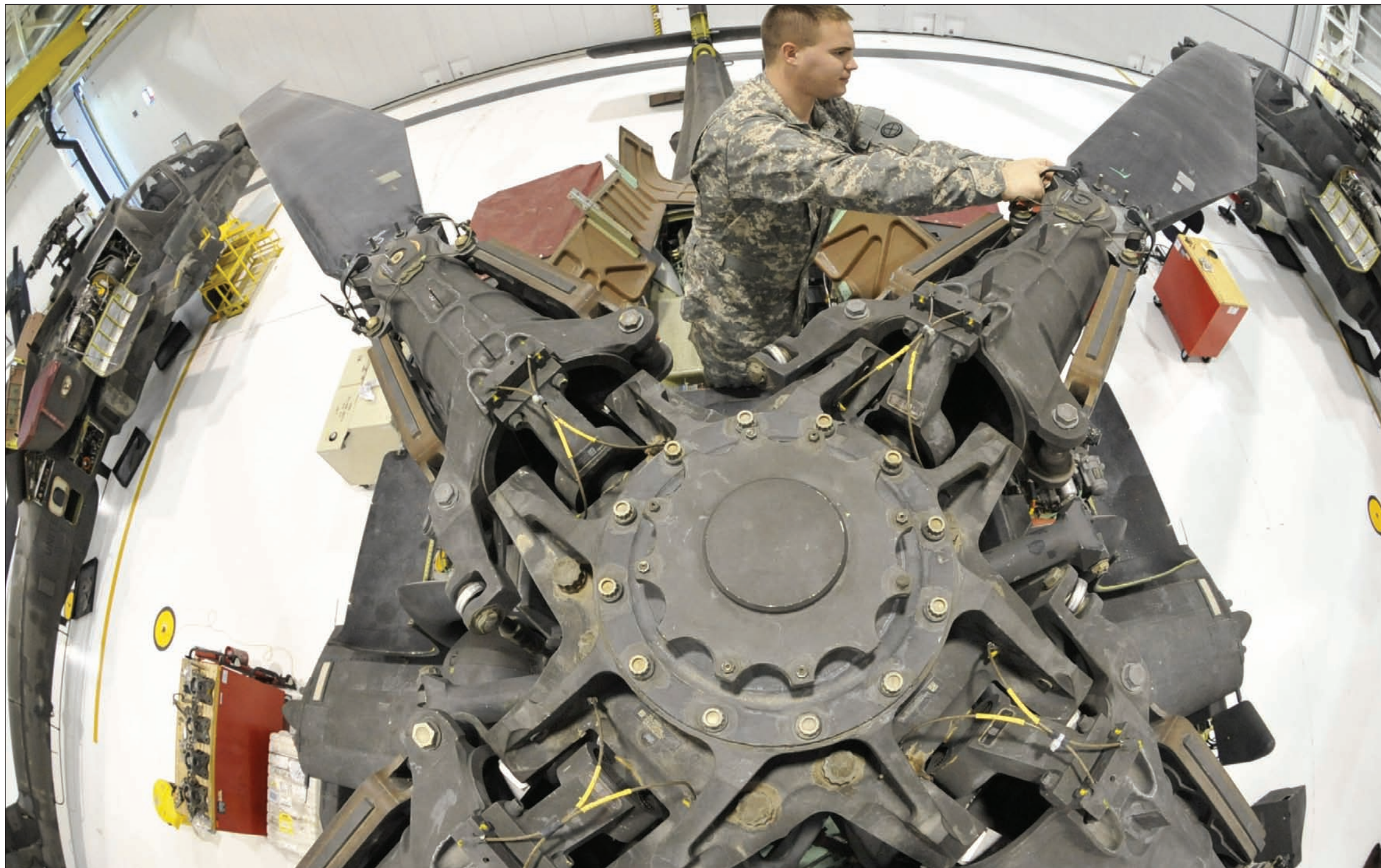
U.S. Army Spc. Todd Gann, 1-135th Attack/Reconnaissance Battalion aircraft maintainer, inspects the main rotor head of an AH-64 Apache at Whiteman Air Force Base, Mo., Jan. 9, 2014. Soldiers perform this inspection annually to ensure there are no signs of corrosion developing, which could cause malfunctions.
