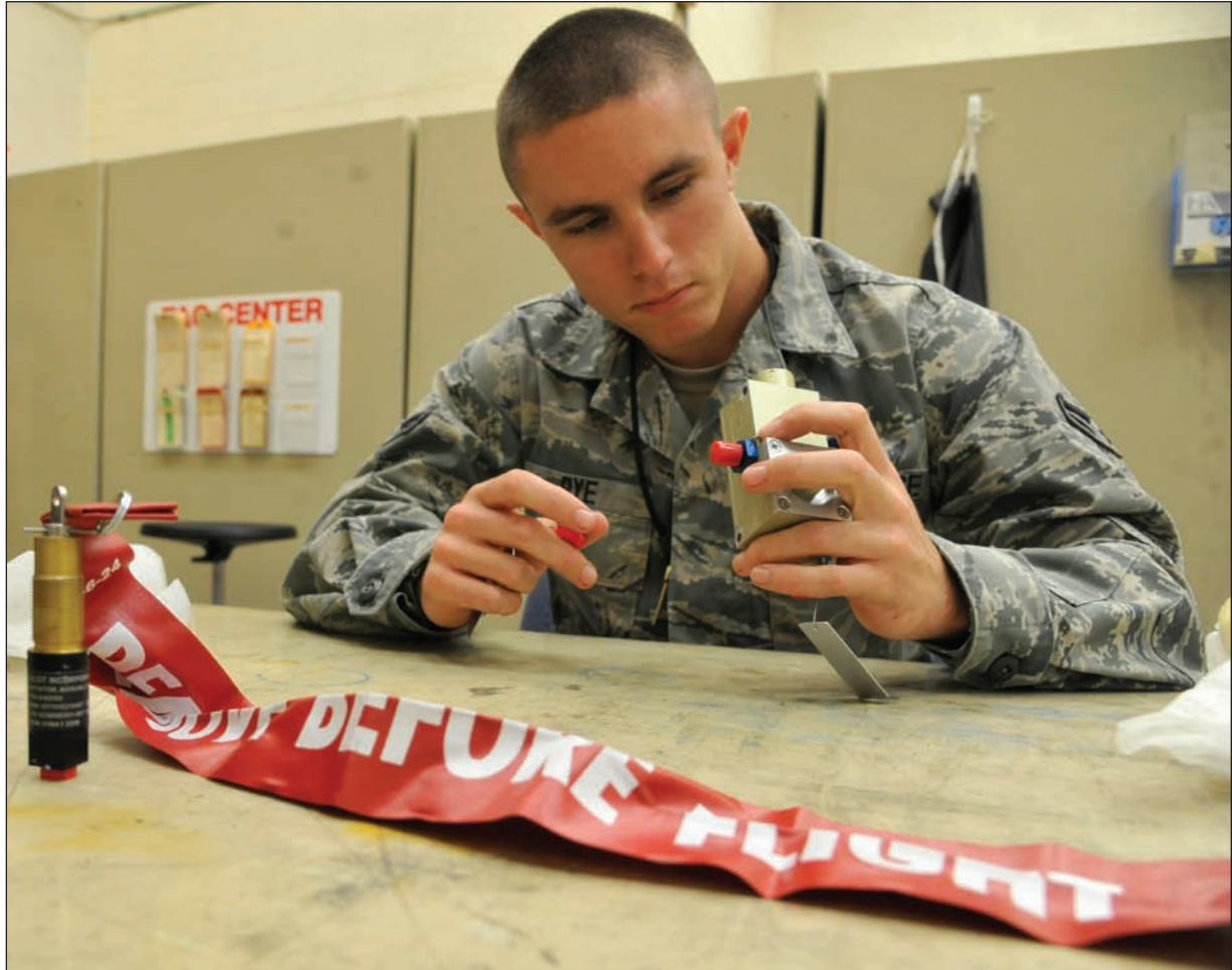
U.S. Air Force Airman 1st Class Justin Rye, 509th Maintenance Squadron egress shop apprentice, inspects a pressure delay initiator (PDI) at Whiteman Air Force Base, Mo., Oct. 22, 2013. The PDI detects the air pressure difference inside the cockpit and outside the aircraft during the ejection sequence. Once the desired range is achieved, the ejection sequence will continue to hatch removal.
