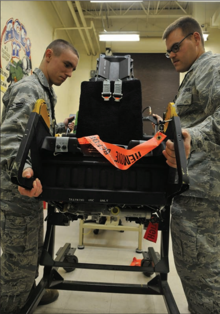
U.S. Air Force Airman 1st Class Justin Rye, right, 509th Maintenance Squadron egress shop apprentice, and U.S. Air Force Staff Sgt. Todd Branthoover, 509th MXS egress swing shift leader, tilt an ACES II ejection seat at Whiteman Air Force Base, Mo., Oct. 28, 2013. Tilting the ACES II seat enables techs to perform time changes and maintenance procedures.
