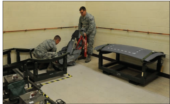
U.S. Air Force Airman 1st Class Justin Rye, right, 509th Maintenance Squadron egress shop apprentice, and U.S. Air Force Staff Sgt. Todd Branthoover, 509th MXS egress swing shift leader, lift a T-38 ejection seat at Whiteman Air Force Base, Mo., Oct. 28, 2013. In the event of an emergency, the ejection seat launches pilots 35 feet into the air.
