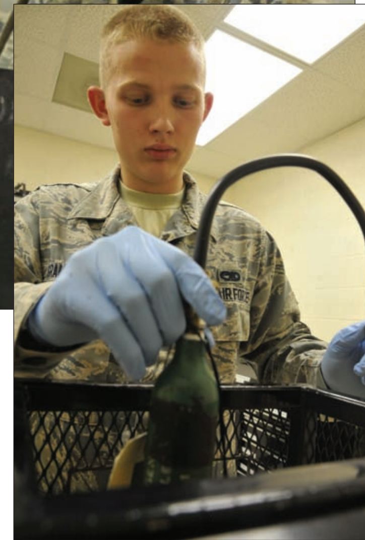
U.S. Air Force Airman 1st Class Chad Grauerholz, 509th Maintenance Squadron electrical environment technician, connects a servicing hose to an emergency oxygen cylinder at Whiteman Air Force Base, Mo., Oct. 15, 2013. The emergency oxygen cylinders are used in the event a pilot needs to eject from an aircraft, providing him or her with ten minutes of oxygen while descending.
