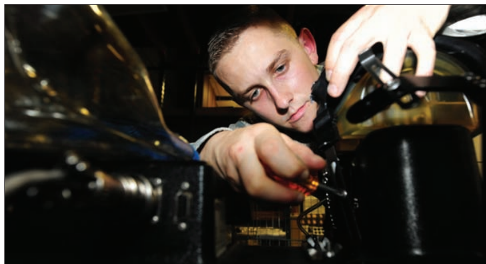
U.S. Air Force Airman 1st Class David Reddoch, 509th Logistics Readiness Squadron individual protective equipment technician, uses a joint-service mask leakage tester (JSMLT) to ensure proper fit of a gas mask as part of a routine inspection at Whiteman Air Force Base, Mo., July 29, 2013. In addition to testing gas masks, IPE technicians are trained on a variety of tasks, including the operation of heavy equipment, customer service and maintenance and accountability of more than 211,000 IPE items valued at approximately $9 million.
