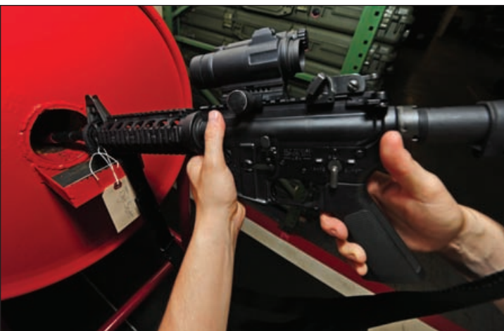
U.S. Air Force Airman 1st Class David Reddoch, 509th Logistics Readiness Squadron individual protective equipment technician, clears an M4 carbine before beginning cleaning procedures at Whiteman Air Force Base, Mo., July 29, 2013. Weapons-clearing procedures include ensuring weapons are set to safe and the chamber is clear of any bullets.
