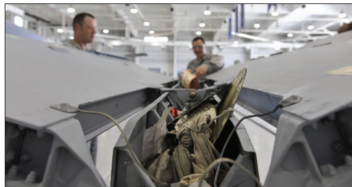
Tech. Sgt. Michael Schuler, 442nd Maintenance Squadron phase dock technician, and Tech. Sgt. Brandon Thompson, 442nd MXS phase dock coordinator, route the hydraulic lines of a speed brake actuator on an A-10 Thunderbolt II at Whiteman Air Force Base, Mo., June 11, 2013. Thompson is performing a clearance check, ensuring the lines are not rubbing against each other or air frame components, which could cause short-circuiting.
