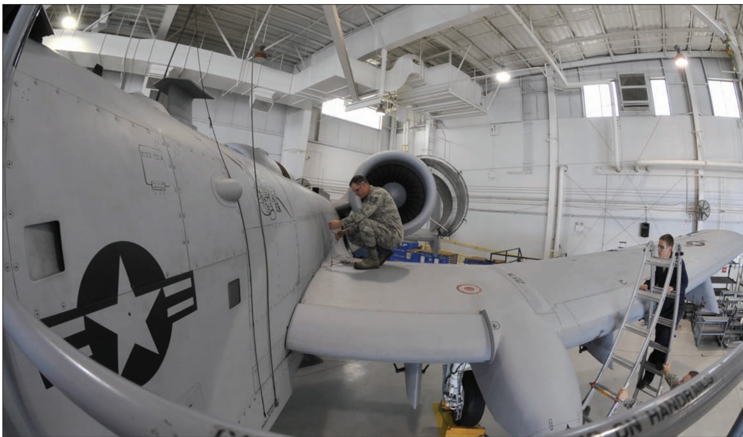
Tech. Sgt. Michael Schuler, 442nd Maintenance Squadron phase dock technician, removes panel F-83 off an A-10 Thunderbolt II at Whiteman Air Force Base, Mo., June 11, 2013. Removing this panel enables maintenance techs to inspect the A-10 and locate any internal discrepancies.
