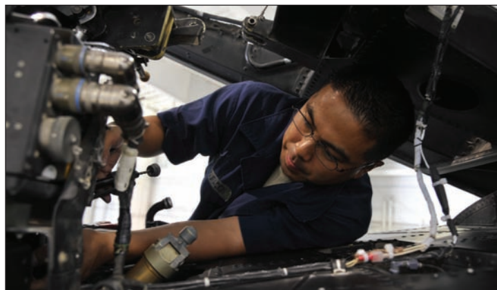
Tech. Sgt. Rodney Transfiguracion, 442nd Maintenance Squadron repair and reclamation technician, repairs canopy closing mechanisms on an A-10 Thunderbolt II at Whiteman Air Force Base, Mo., June 11, 2013. Transfiguracion is working to determine why this particular canopy is not locking; the canopy must lock to ensure the pilot is safe and secure in the cockpit.
