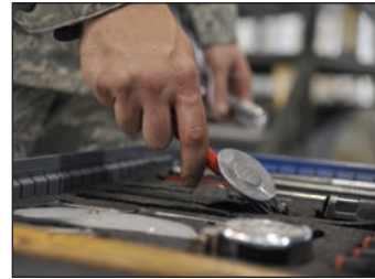
Tech. Sgt. Michael Schuler, 442nd Maintenance Squadron phase dock technician, grabs a round mirror and flashlight for an A-10 Thunderbolt II engine inspection at Whiteman Air Force Base, Mo., June 11, 2013. The mirror helps technicians see into spaces of the jet too tight to look into directly and the flashlight is used to illuminate areas within engines, panels and wheel wells.
