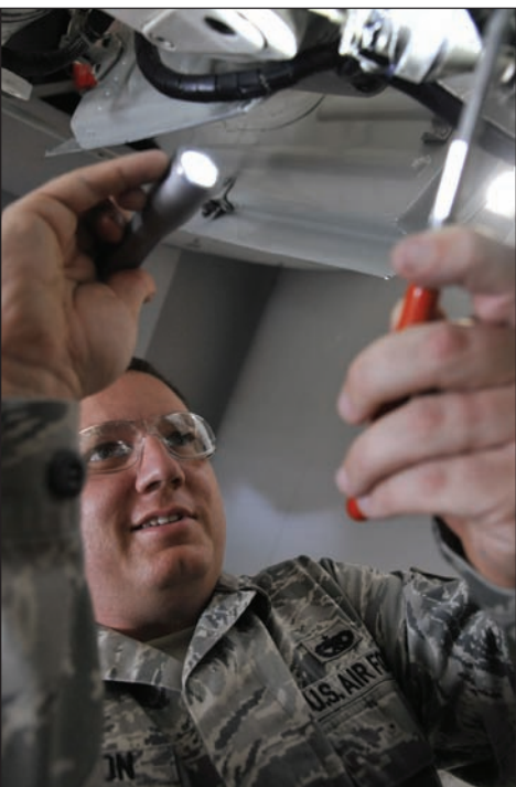
Tech. Sgt. Brandon Thompson, 442nd Maintenance Squadron phase dock coordinator, inspects a weight-on-wheels switch on the left main landing gear of the A-10 Thunderbolt II at Whiteman Air Force Base, Mo., June 11, 2013. This is a required inspection item, and ensures the drain hole is properly positioned.
