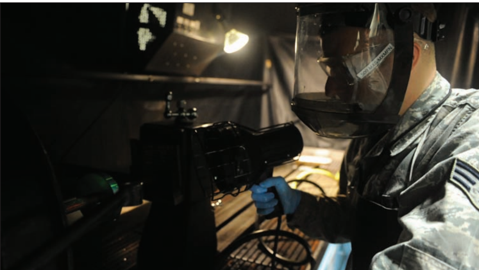
Senior Airman Joel Flowers, 509th Maintenance Squadron non-destructive inspection journeyman, uses a black light to inspect an aircraft part at Whiteman Air Force Base, Mo., May 1, 2013. The black light causes particles normally unseen by the human eye to become florescent.
