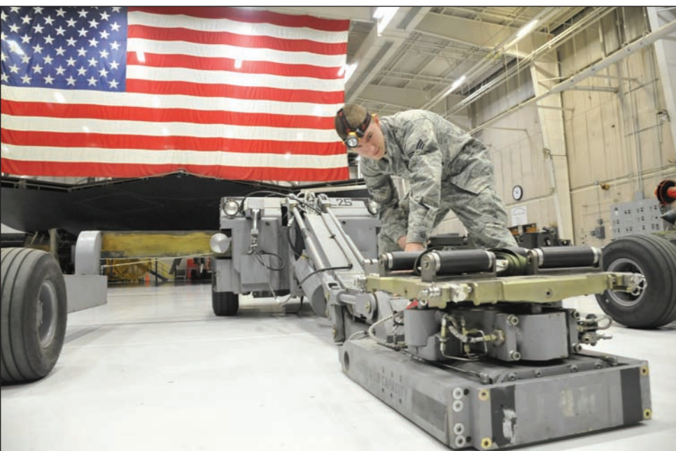
U.S. Air Force photo/Airman 1st Class Keenan Berry Senior Airman Charles Balog, 509th Aircraft Maintenance Squadron weapons loader, examines a rotary launcher assembly (RLA) before beginning a weapons load demonstration at Whiteman Air Force Base, Mo., May 3, 2013. Balog is training for real-life scenarios that could require him and his fellow weapons team to rapidly and securely load munitions into the B-2 using this and other machinery.
