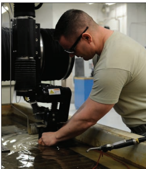
U.S. Air Force Tech. Sgt. Jim Gargano, 509th Maintenance Squadron metals technology assistant section chief, uses a water jet machine to cut pieces of metal for aircraft parts, March 6. Water jets do not leave heat-affected zones, generate noxious fumes or create mechanical stresses on the surfaces of the cut piece.
