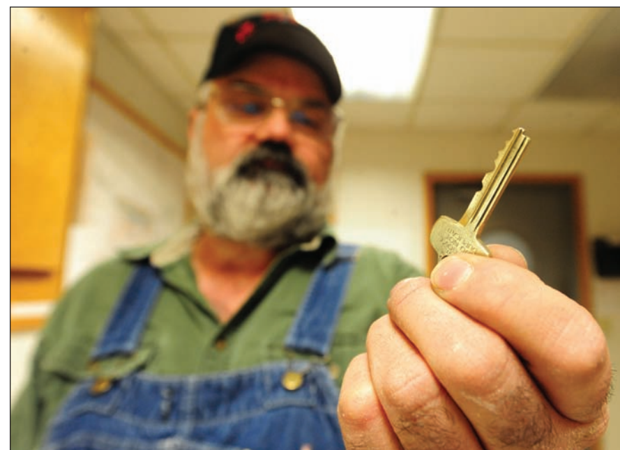
Jack Crain, 509th Civil Engineer Squadron locksmith, inspects a key for precision after cutting it, March 6. The depth and spacing of the grooves of keys locksmiths cut must be correct down to a thousandth of an inch or the key will not work.
