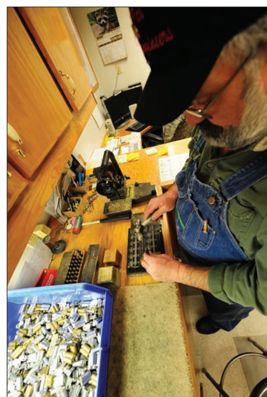
Jack Crain, 509th Civil Engineer Squadron locksmith, hammers pinning codes into a key, March 6. Different series of numbers help prevent the duplication of keys and maintain the continuity of locks.
