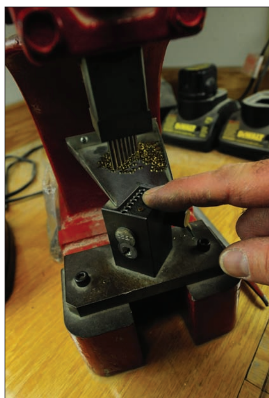
Jack Crain, 509th Civil Engineer Squadron locksmith, inspects the holes of a lock before pressing caps into the lock core, March 6. Without the caps, the lock will never be secure.
