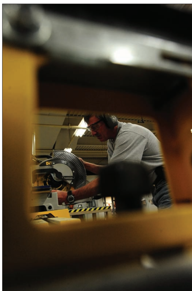
Albert Cote, 509th Civil Engineer Squadron carpenter, cuts a piece of wood for a door frame with a compound miter saw, Feb. 27. Cote works with a team of professionals responsible for performing all aspects of carpentry and masonry, including sheet metal, wood and welding work.
