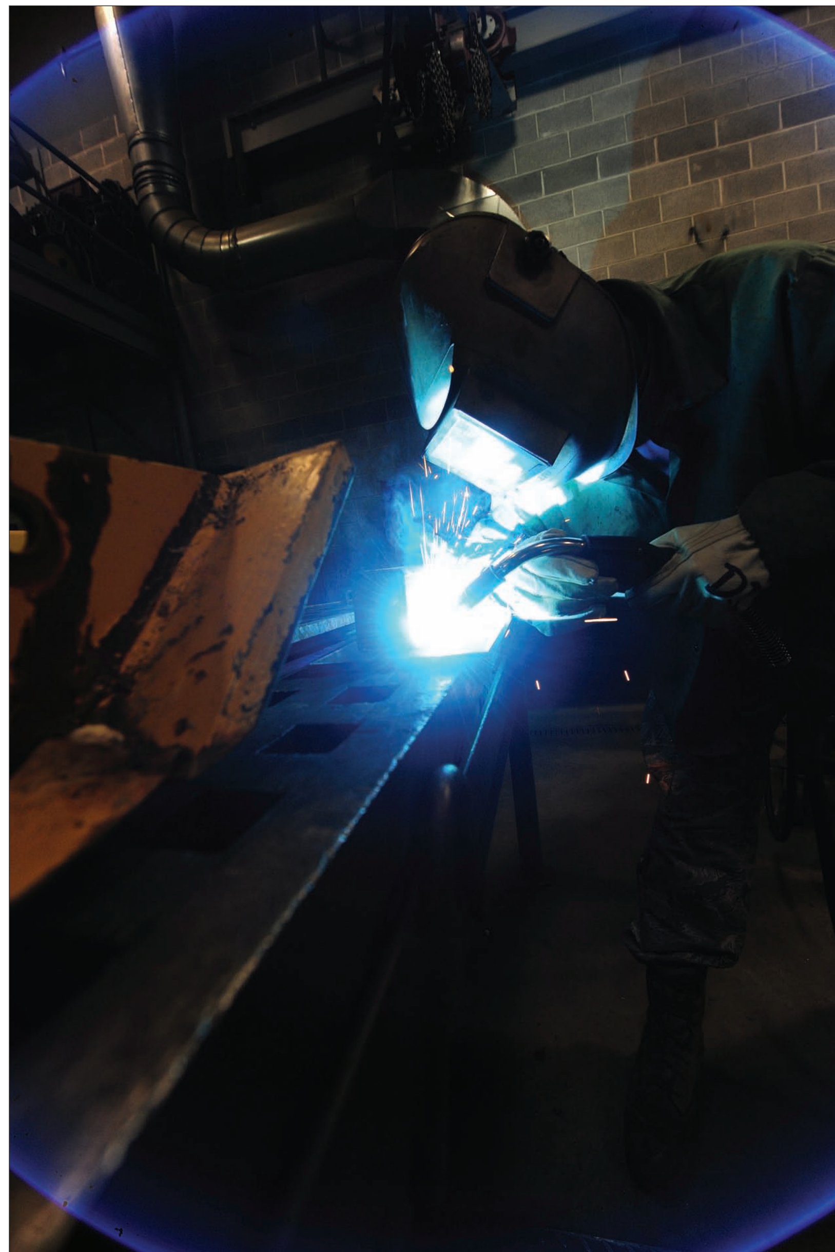
Senior Airman Michael Rafael, 509th Civil Engineer Squadron structural journeyman, welds a box blade for a snow plow, Feb. 27. Structural journeymen are responsible for maintaining knowledge and proficiency in metal layout, metal fabrication, welding, cutting, brazing and locksmithing.
