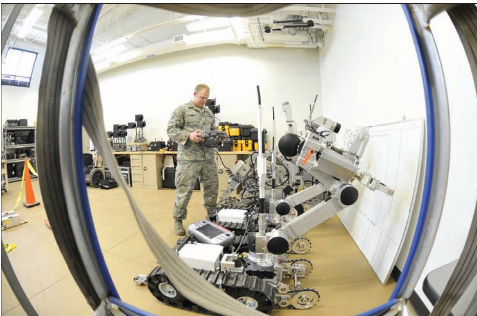
Airman 1st Class Jeff Kinney, 509th Civil Engineer Squadron Explosive Ordnance Disposal team member, performs a function check on the AFMSR and the F-6 robot, Feb. 27. These robots are both designed to destroy improvised explosive devices.
