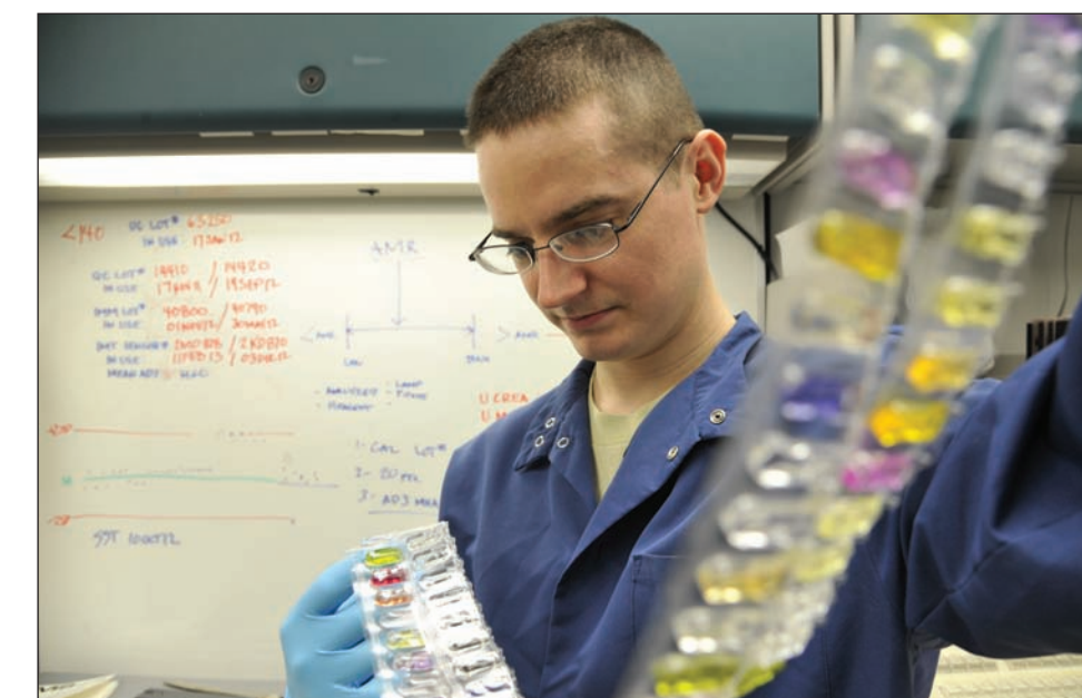
Staff Sgt. Nathan Knox, 509th Medical Group medical laboratory scientist, examines a set of cuvettes, Feb. 20. The cuvettes are designed to contain medical samples, and are examined by a chemistry analyzer to determine what a person's test value is based off of color changes.
