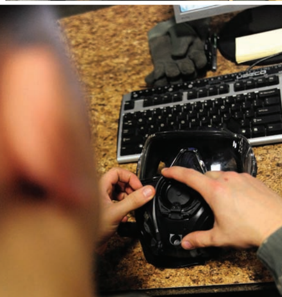
Airman 1st Class Jonathan Merry, 509th Logistics Readiness Squadron individual protective equipment technician, tests the fitting of a gas mask to ensure the valves have a proper seal, Feb. 7. A loose seal could mean the difference between life and death for an Airman under a chemical attack, according to Merry.
