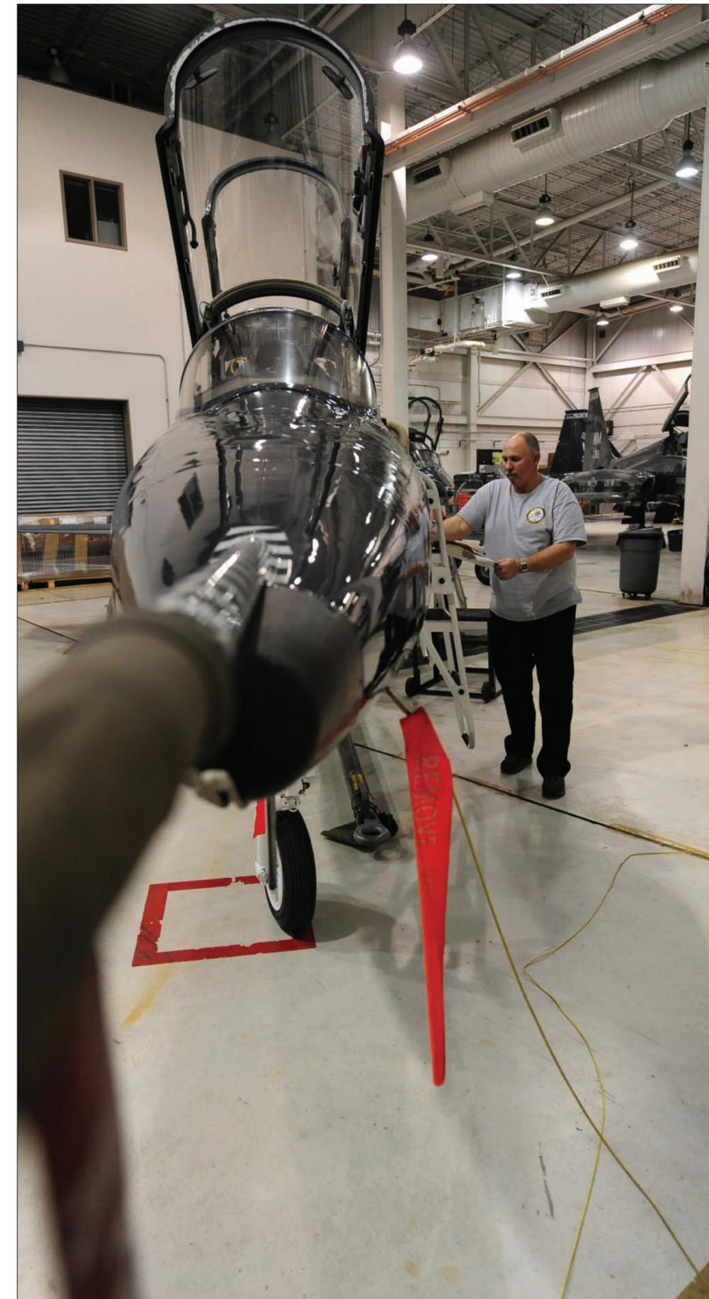
Russ Cass, M1 Support Services aircraft mechanic, processes aircraft forms on a T-38 Talon, Jan. 24. Aircraft forms are used to document maintenance being performed, malfunctioning components and aircraft status.
