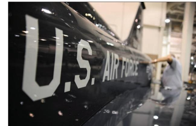
Russ Cass, M1 Support Services aircraft mechanic, secures an access panel for a hydraulic reservoir on a T-38 Talon, Jan. 24. These panels enable mechanics to more easily access the aircraft and perform repairs on various components.
