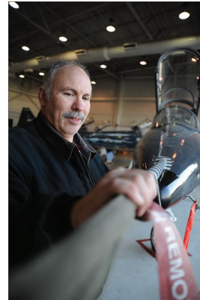
Russ Cass, M1 Support Services aircraft mechanic, uses a pitot tube cover to screen an aircraft before “putting the aircraft to bed,” Jan 23. In maintenance terms, this phrase means the aircraft is being secured for the evening after the flying day.
