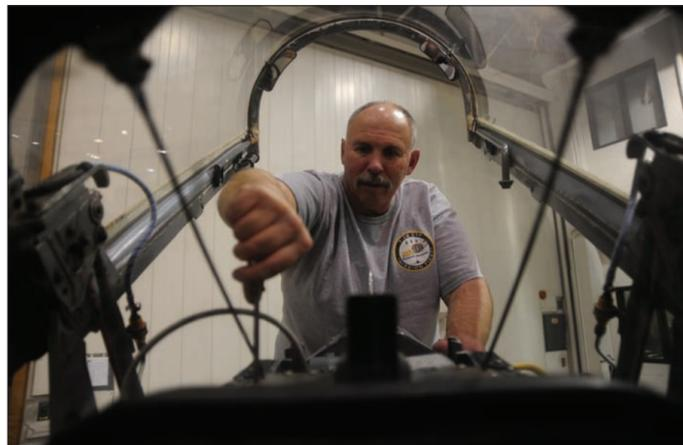
Russ Cass, M1 Support Services aircraft mechanic, checks the tightness of a screw on an ejection seat in a T-38 Talon, Jan. 24. The ejection seat is rocket-powered to allow pilots to escape the aircraft in case of an emergency.
