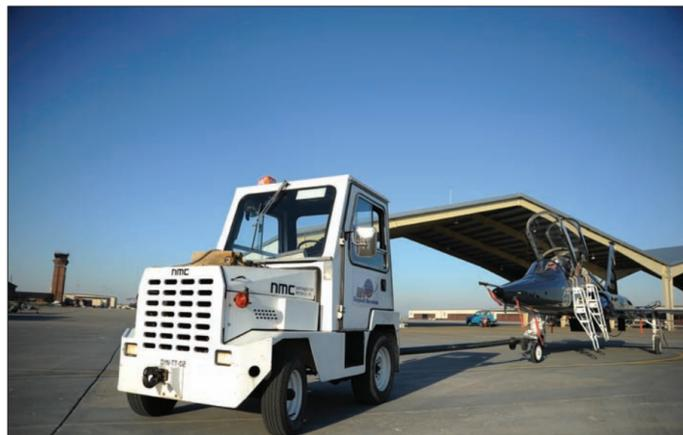
A Warehouse tug is used to tow a T-38 Talon after flight, Jan. 23. Warehouse tugs are used to tow aircraft that weigh 15, 000 pounds or less.
