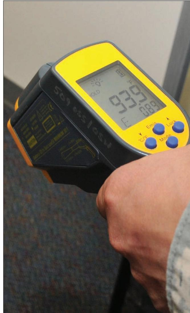
Tech. Sgt. Ryan Watts, 509th Operations Support Squadron, demonstrates an infrared temperature gun during his shift Sept. 13. The Weather Flight uses the device to take temperature readings and is primarily used in the winter to determine the rate at which snow melts.
