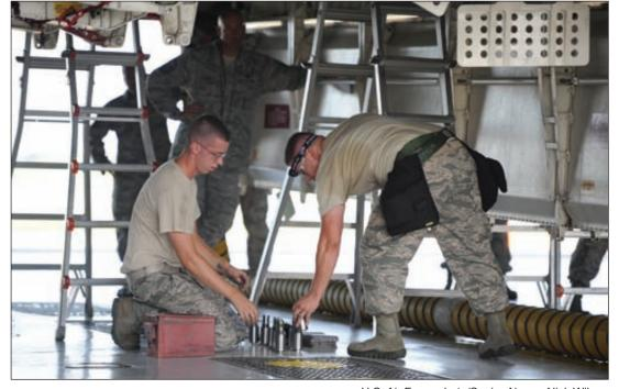
Airmen from the 509th Aircraft Maintenance Squadron prepare to place impulse cartridges into the bomb racks of a B-2 Spirit during an Air Force Global Strike Command Weapons Load competition, Sept. 6. The purpose of each cartridge is to create an electrical charge which causes the bomb rack to unlock so munitions can be released.
