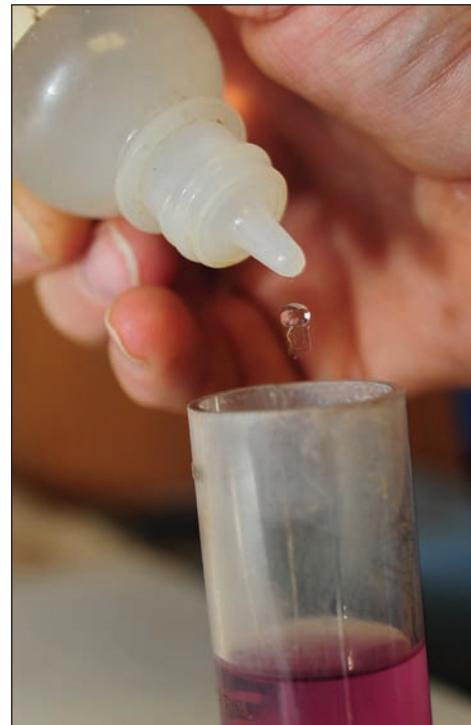
Paul Ross, 509th Civil Engineer Squadron central heat plant project manager, performs a boiler chemistry test to verify water used by the base's heat plant is clean and ready for use, Aug. 27. Maintaining proper chemistry in boiler water prevents deterioration and corrosion of pipes that carries the heat plant's water.
