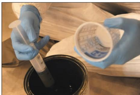
(ABOVE/RIGHT) Airman 1st Class Mathew Wert, 509th Maintenance Squadron low observable technician, measures paint for the B-2 Spirit coating. The LO section maintains the stealth capabilities of the B-2 by repairing the LO coating and internal and external structural hardware.
