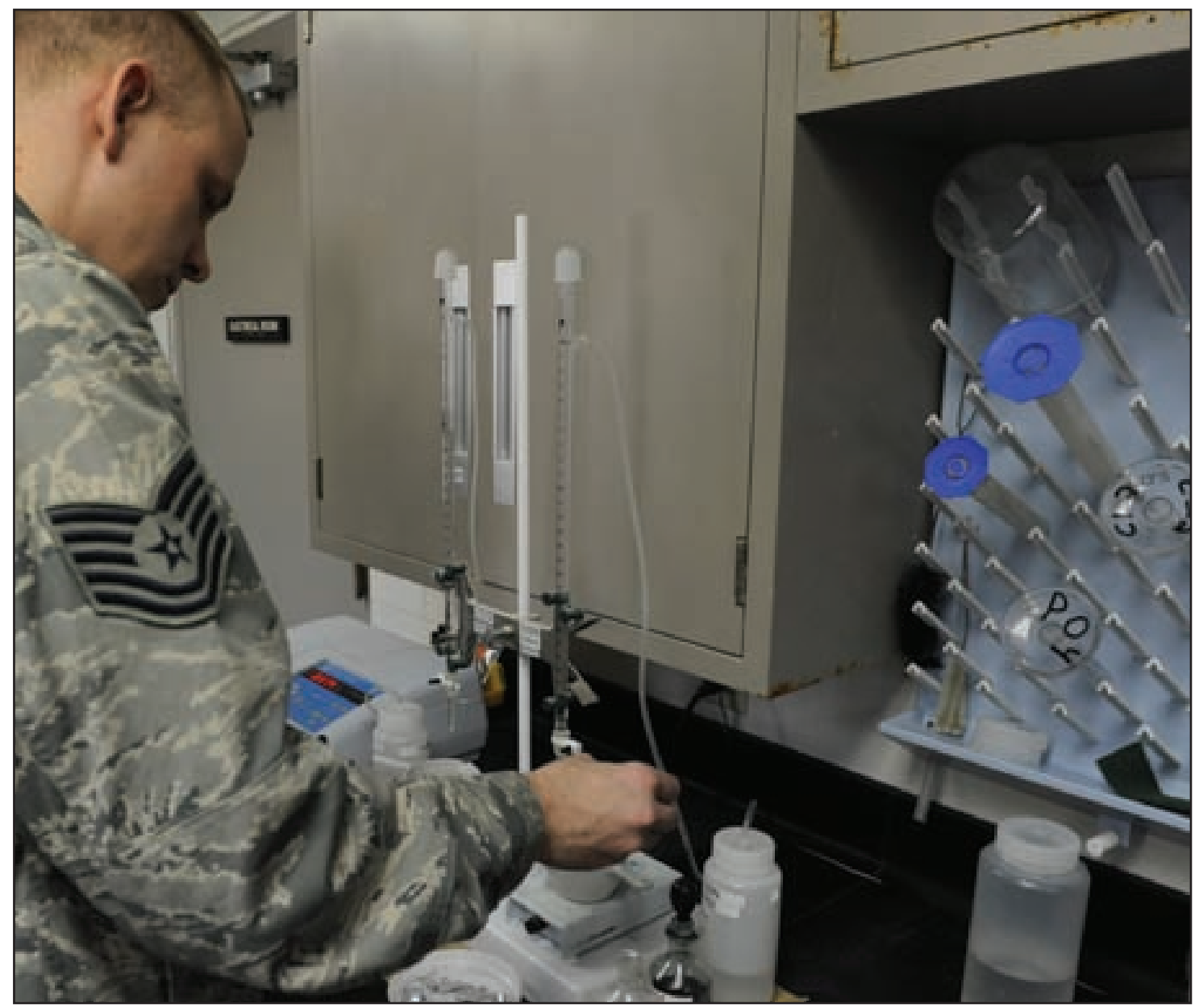
Tech. Sgt. Jason Jenkins, 509th Civil Engineer Squadron water fuels systems supervisor, runs a water hardness test at the water treatment plant Jan. 19. The water treatment facility softens 220 million gallons of water per year to reduce the hardness which in turn extends the longevity of the base infrastructure.
