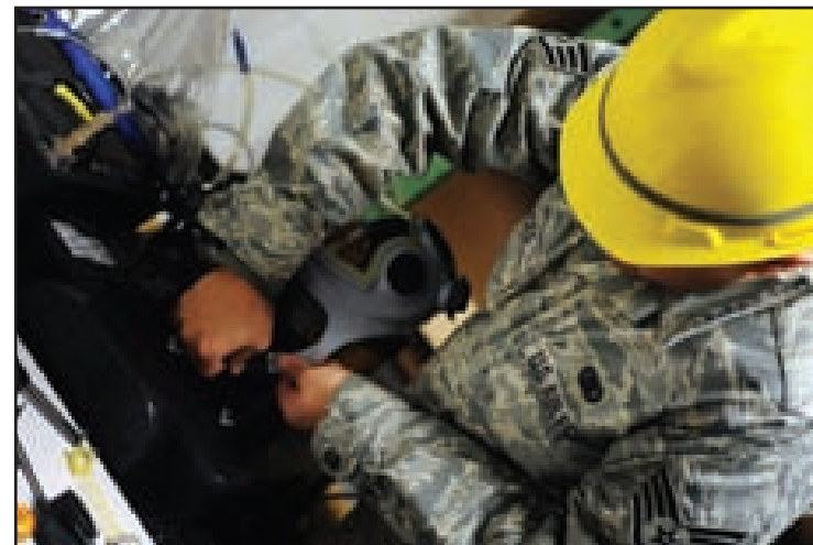
(TOP) Staff Sgt. Justin Garcés, 509th LRS, buckles down a MCU-2/P series protective mask to be tested. (BOTTOM) MCU-2/P series protective masks hang from a wash rack after being soaked in solution.
