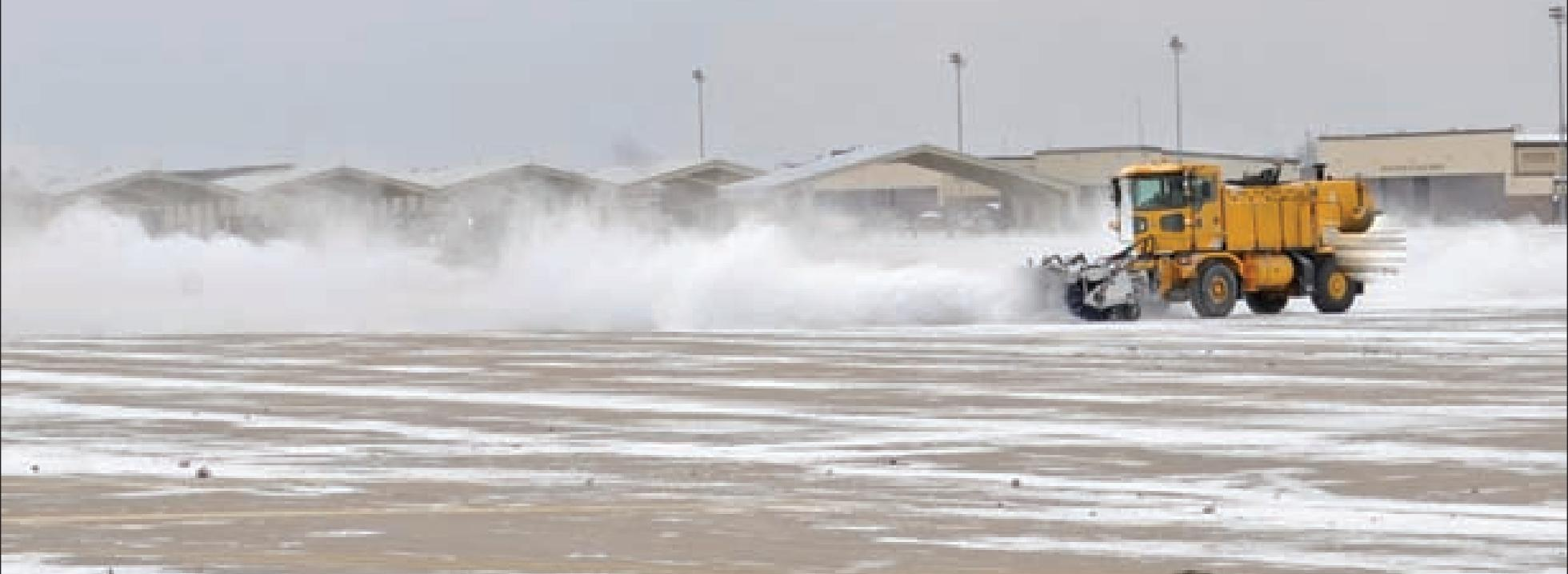
The 509th Civil Engineer Squadron shovels snow off the flightline Jan. 12. Clearing the flightline for aircraft requires the use of heavy equipment. An 18-foot-wide snow broom, 20-foot-wide plow and 54,000-pound roll-over plow allow the airfield to be cleared in a timely manner.
