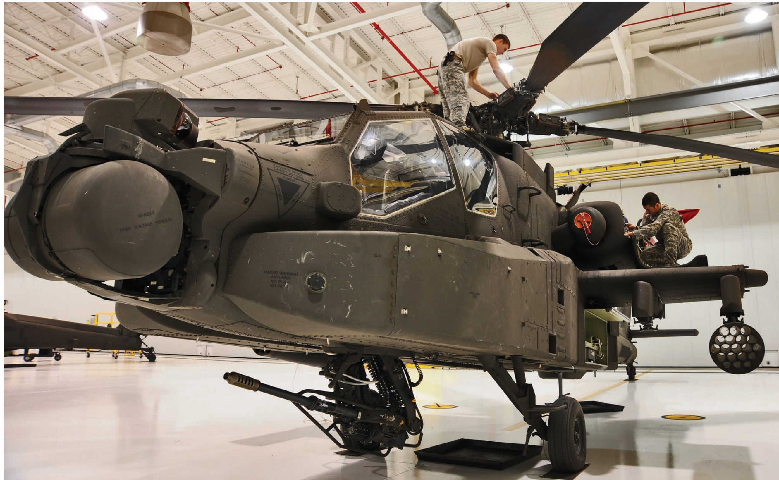
ALL PHOTOS: Soldiers from the 1-135th Attack Reconnaissance Battalion perform maintenance on an AH-64D Apache Longbow Nov. 23. Each Longbow goes through a phase inspection every 500 flight hours, where major components of the aircraft are inspected and fixed.
