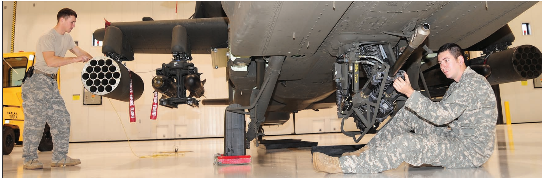
ALL PHOTOS: Soldiers from the 1-135th Attack Reconnaissance Battalion perform maintenance on an AH-64D Apache Longbow Nov. 23. Each Longbow goes through a phase inspection every 500 flight hours, where major components of the aircraft are inspected and fixed.
