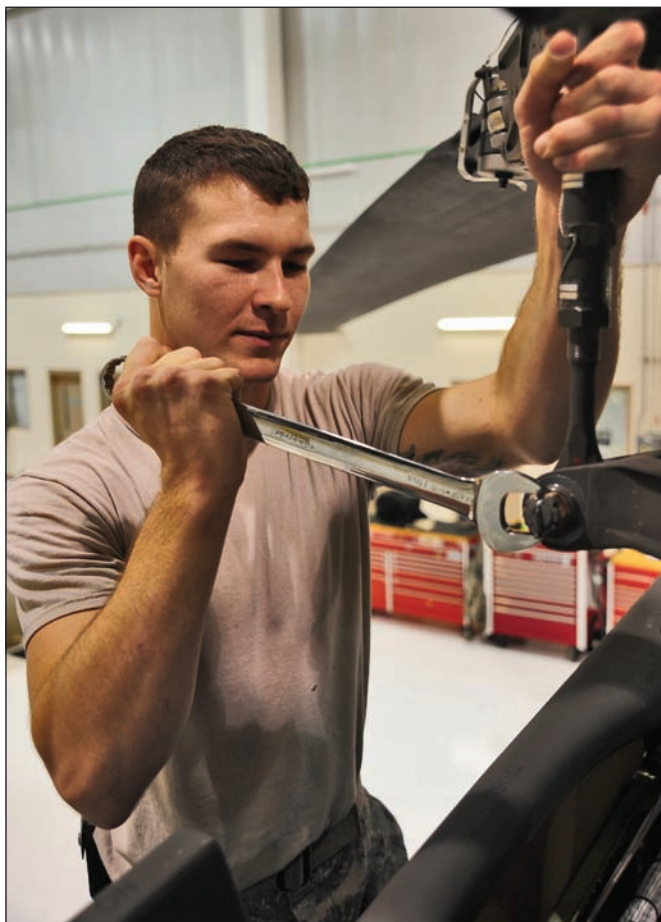
ALL PHOTOS: Soldiers from the 1-135th Attack Reconnaissance Battalion perform maintenance on an AH-64D Apache Longbow Nov. 23. Each Longbow goes through a phase inspection every 500 flight hours, where major components of the aircraft are inspected and fixed.
