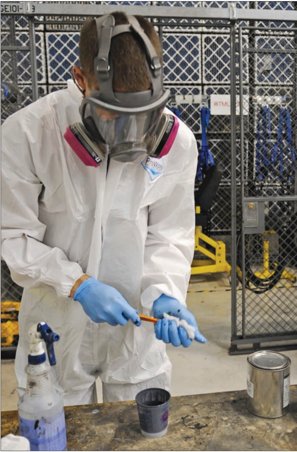
Senior Airman Kyle Miller, 509th Maintenance Squadron B-2 Spirit LO structural maintenance technician, mixes chemicals to produce the top coat for visual purposes here July 8. The LO section maintains the stealth capabilities of the B-2 by repairing the LO coating and internal and external structural hardware.
