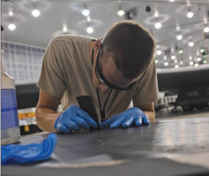
Senior Airman Kyle Miller, 509th Maintenance Squadron B-2 Spirit LO structural maintenance technician, removes the coating on the B-2 here July 8. The LO characteristics of the B-2 are a means of defense this aircraft has during combat missions.
