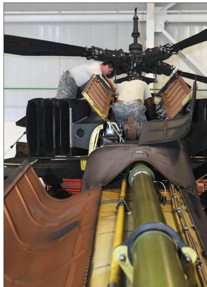
U.S. Air Force photo by Senior Airman Alexandra M. Boutte Staff Sgt. Ryan Cody and Sgt. 1st Class Andrew Butler, 1-135 Attack Reconnaissance Battalion aircraft maintainers, inspects a Boeing AH-64 Apache helicopter here May 31. The Apache features double and triple-redundant avionics systems to improve survivability for the aircraft and crew in combat.
