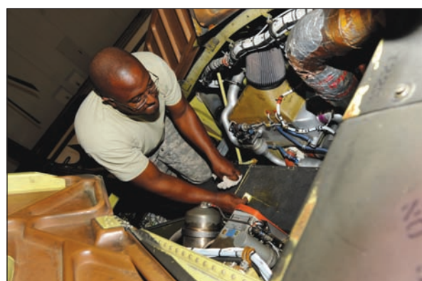
U.S. Air Force photo by Senior Airman Alexandra M. Boutte Sgt. 1st Class Andrew Butler, 1-135 Attack Reconnaissance Battalion aircraft maintainer, hooks up vibration cables to the transmission of a Boeing AH-64 Apache helicopter here May 31. The vibration cables are fastened to the transmission to ensure the transmission is working properly.
