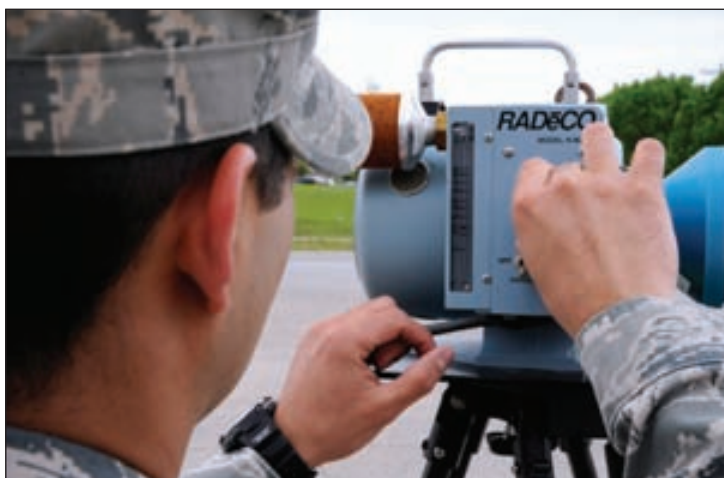
Staff Sgt. Edwin Origel, 509th Medical Operations Squadron bioenvironmental technician, adjusts air monitoring equipment to sample alpha particles in the air here May 2.
