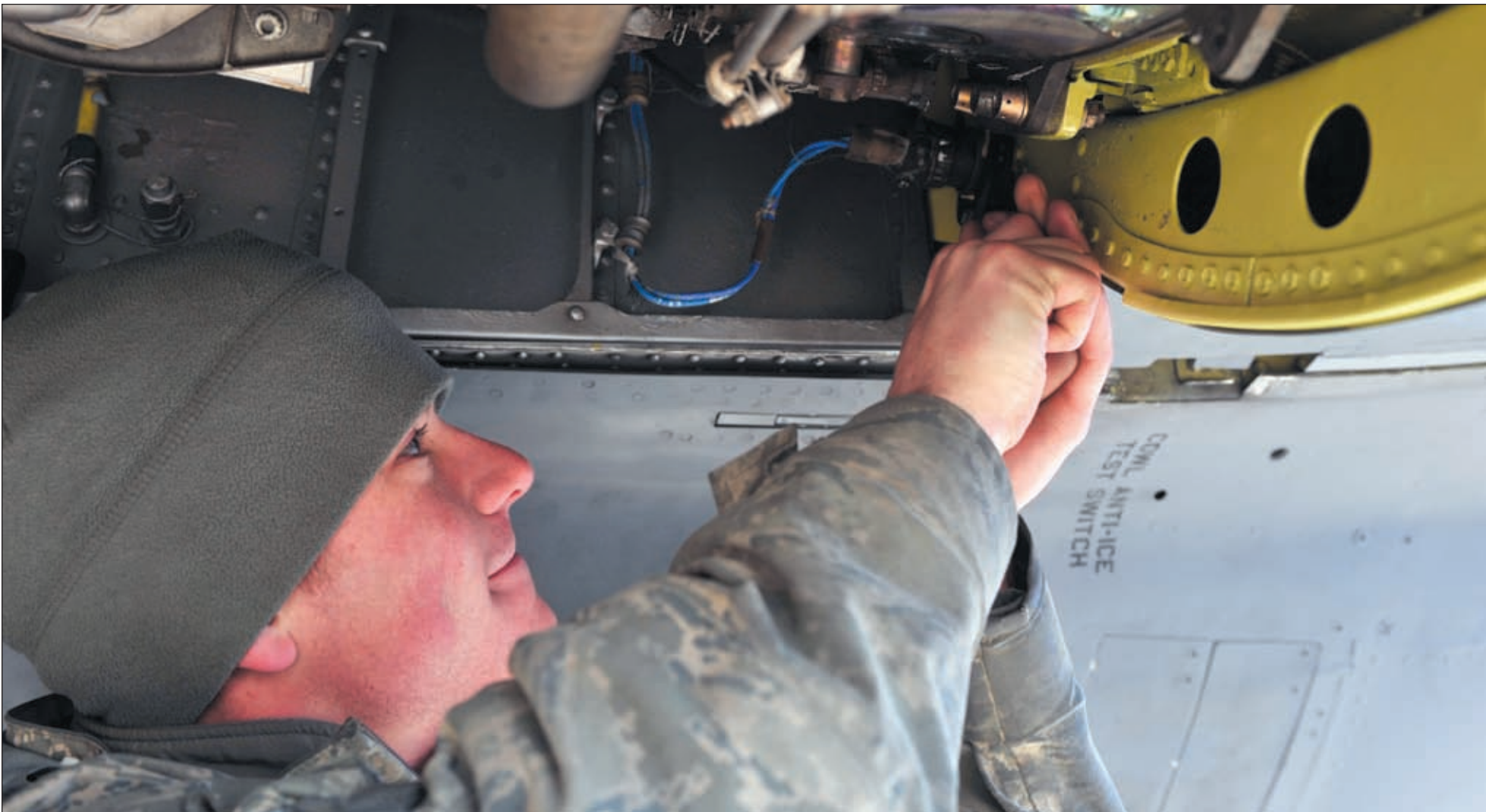
MINOT AIR FORCE BASE, N.D. -- Senior Airman George Querry, 5th Aircraft Maintenance Squadron electrical and environmental specialist, works on the anti-ice system inside the compartment of one of the engines on a B-52H Stratofortress April 1. (U.S. Air Force photo by Staff Sgt. Keith Ballard)
