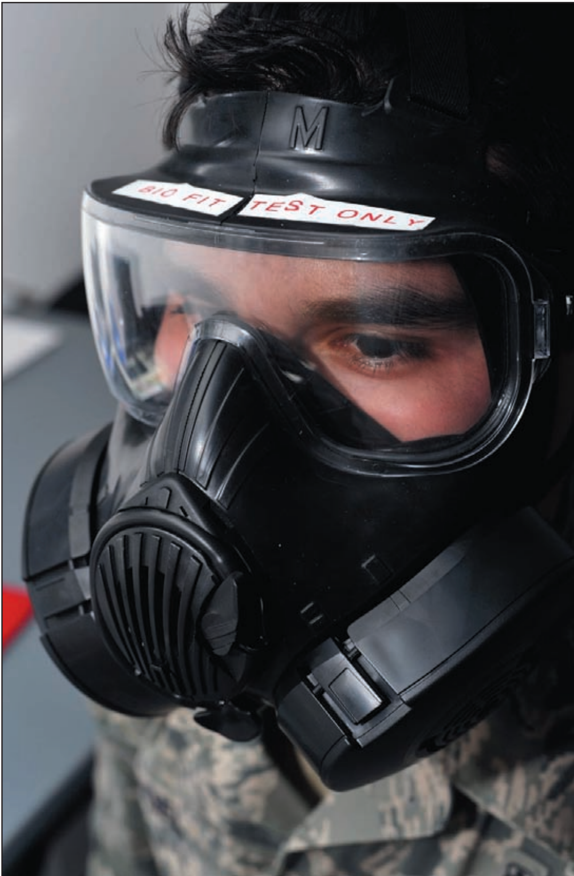
Staff Sgt. Edwin Origel, 509th Medical Support Squadron bioenvironmental engineering technician, demonstrates the procedures for fit testing the new M50 gas mask March 1. Sergeant Origel ran an operational check on the system prior to arrival of the Airmen scheduled for appointments.
