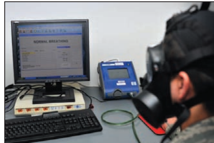
(Photo above and left) Staff Sgt. Edwin Origel, 509th Medical Support Squadron bioenvironmental engineering technician, monitors a fit test system designed to test the new M50 gas mask March 1. Sergeant Origel ran an operational check on the system prior to the arrival of the Airmen scheduled for appointments.
