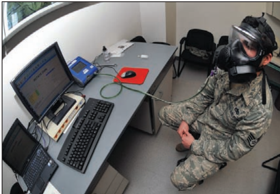
Staff Sgt. Edwin Origel, 509th Medical Support Squadron bioenvironmental engineering technician, demonstrates the procedures for fit testing the new M50 gas mask March 1. Sergeant Origel ran an operational check on the system prior to arrival of the Airmen scheduled for appointments.
