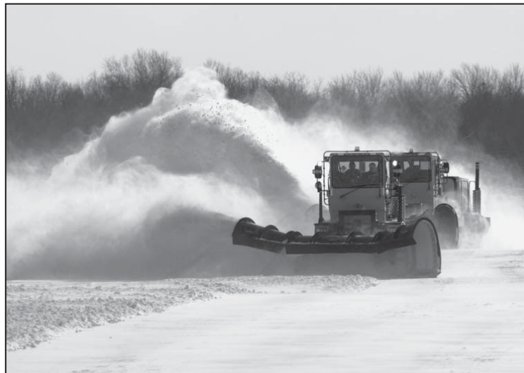
Air Force photo by Senior Airman Jessica No The 509th Civil Engineer Squadron pavements and equipment shop uses 8-foot plows to clear snow off the airfield, an.
