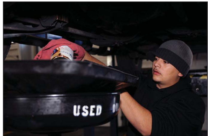
Rey Barajas removes the oil filter from the customer's car as part of the oil change service, Nov 6.
