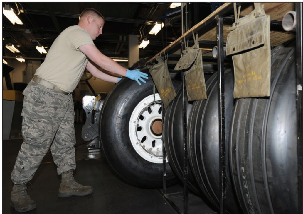
Airman Scott places a finished B-2 main tire assembly into the ready line, Nov. 8. A tire makes it to the ready line after passing the 7-level inspection, which looks over all the work that was completed on the tire and rejects the tire if something was not done correctly.
