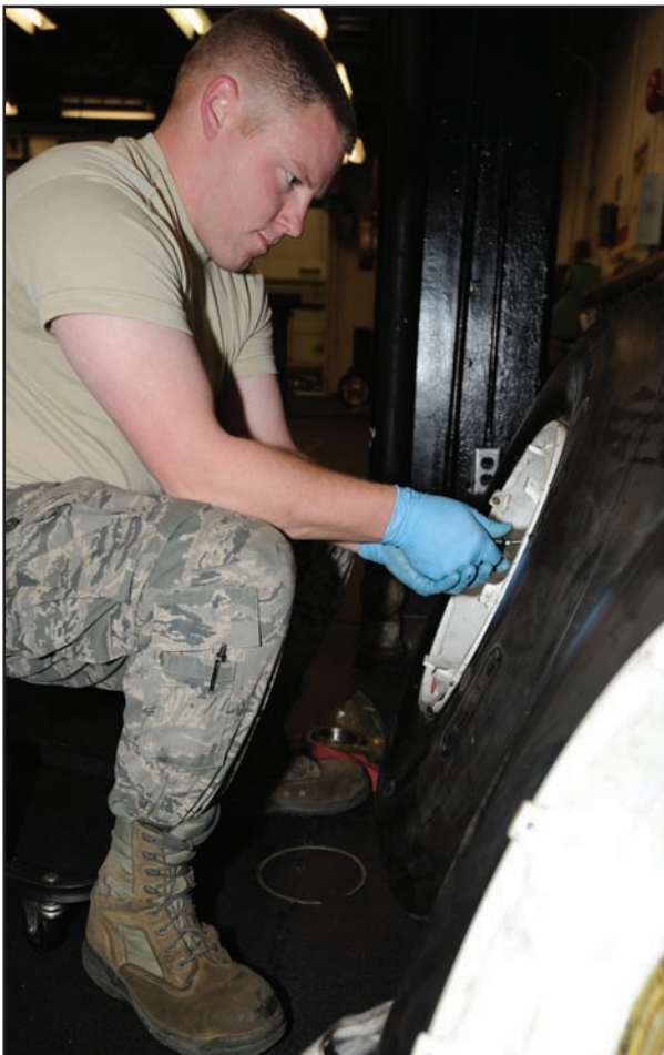
(Above) Airman Scott inserts bearings into a B-2 nose tire, Nov. 8. The wheel and tire shop is responsible for more than 200 B-2 main and nose tires and more than 100 T-38 tires.
