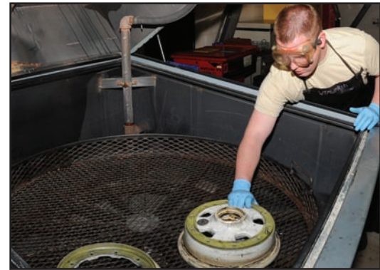
(Above) Airman Scott places two T-38 wheel sections into the automatic washer, Nov. 8. The parts washer is a new piece of equipment to the wheel and tire shop increasing the parts washing efficiency 90 percent. (Left) Airman Scott removes a B-2 nose bolt to be used to attach the split wheel together, Nov. 8. A wheel and tire assembly can take up to two days for completion.
