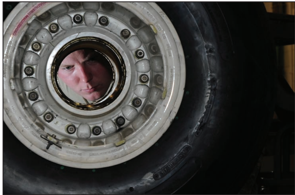
Airman 1st Class Ryan Scott, 509th Maintenance Squadron wheel and tire technician, inspects the B-2 nose tire before it will receive its bearings, Nov.8. The wheel and tire shop inspects each piece of the build intensively, ensuring all steps are followed and the tires are built according to standards.
