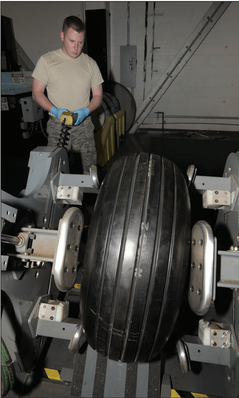
Airman 1st Class Ryan Scott, 509th Maintenance Squadron wheel and tire technician, inspects the B-2 nose tire before it will receive its bearings, Nov.8. The wheel and tire shop inspects each piece of the build intensively, ensuring all steps are followed and the tires are built according to standards.
