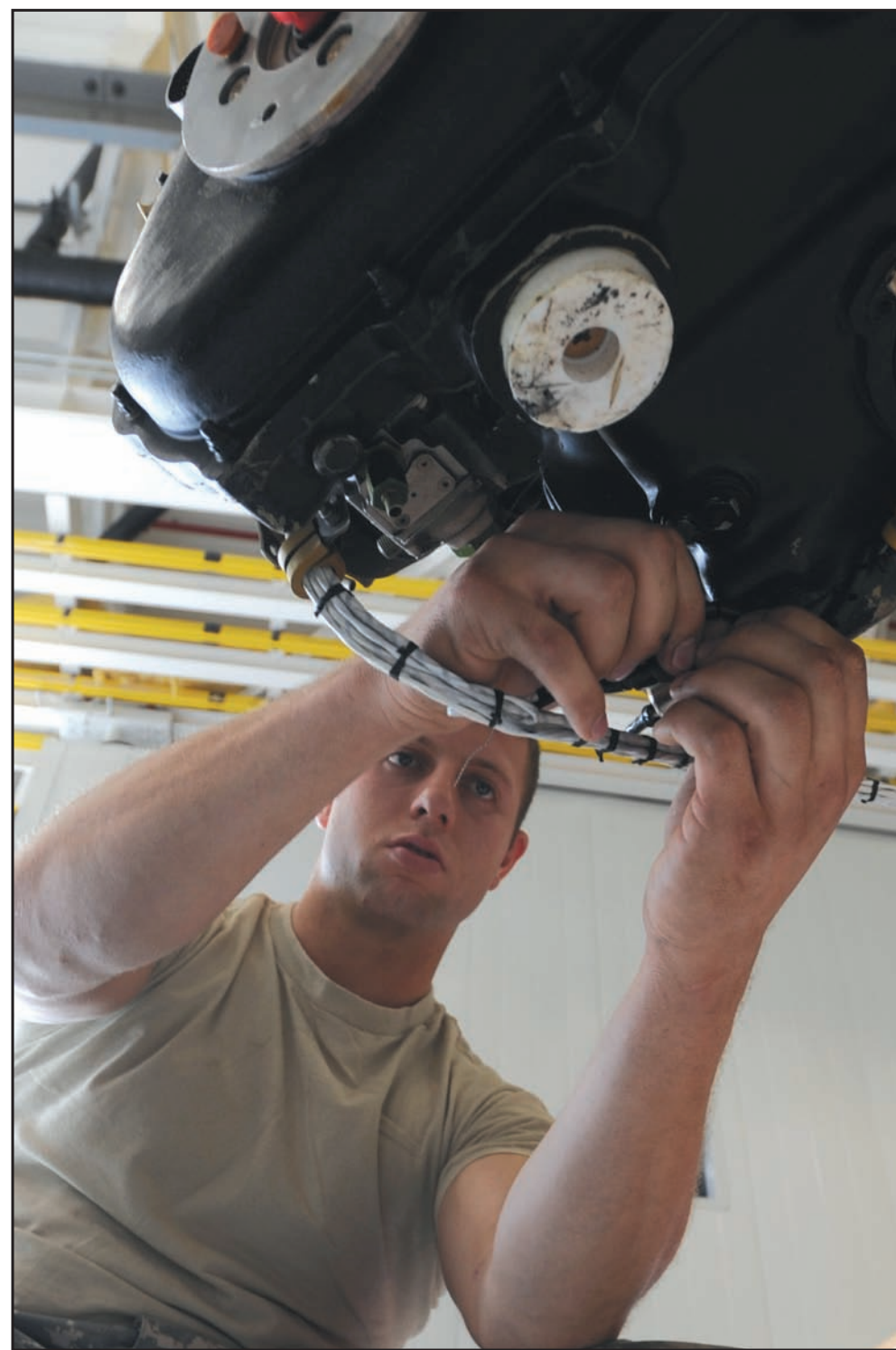
Army Staff Sgt. Jonathan Dalman, 935th Bravo Company Detachment Warrensburg, Mo., maintenance technician, rewires the main rotor drive for an AH-64 Attack Apache Helicopter, Oct. 25. Whiteman Air Force Base is home to the Army Aviation Support facility which maintains the Apache Helicopter when the 1-135th Attack Reconnaissance Battalion is not here for their drill weekend.
