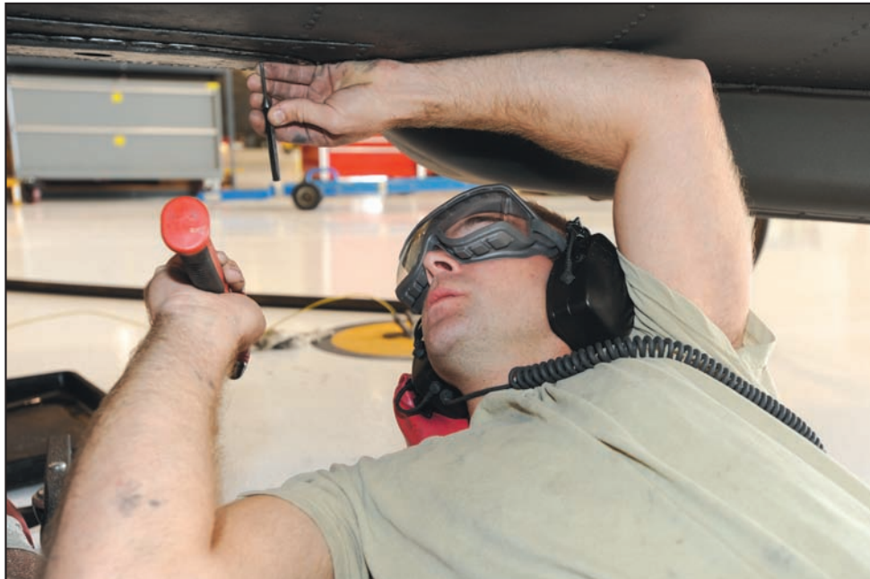
Army Private 1st Class Randall Mayo, 1-135th Attack Reconnaissance Battalion maintenance technician, repairs rivets on the fuselage of an AH-64 Attack Apache, Oct. 26.
