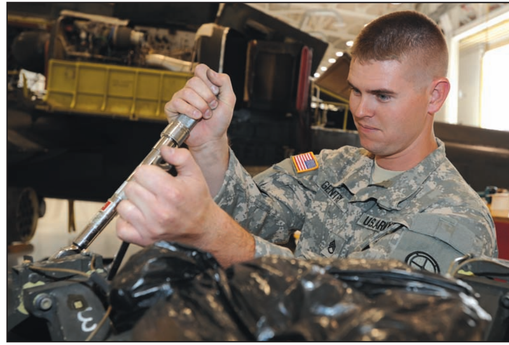
Army Staff Sgt. Brett Gentry, 1-135th Attack Reconnaissance Battalion maintenance technician uses a socket wrench to torque the pitch housing on the main rotor head, Oct. 25.
