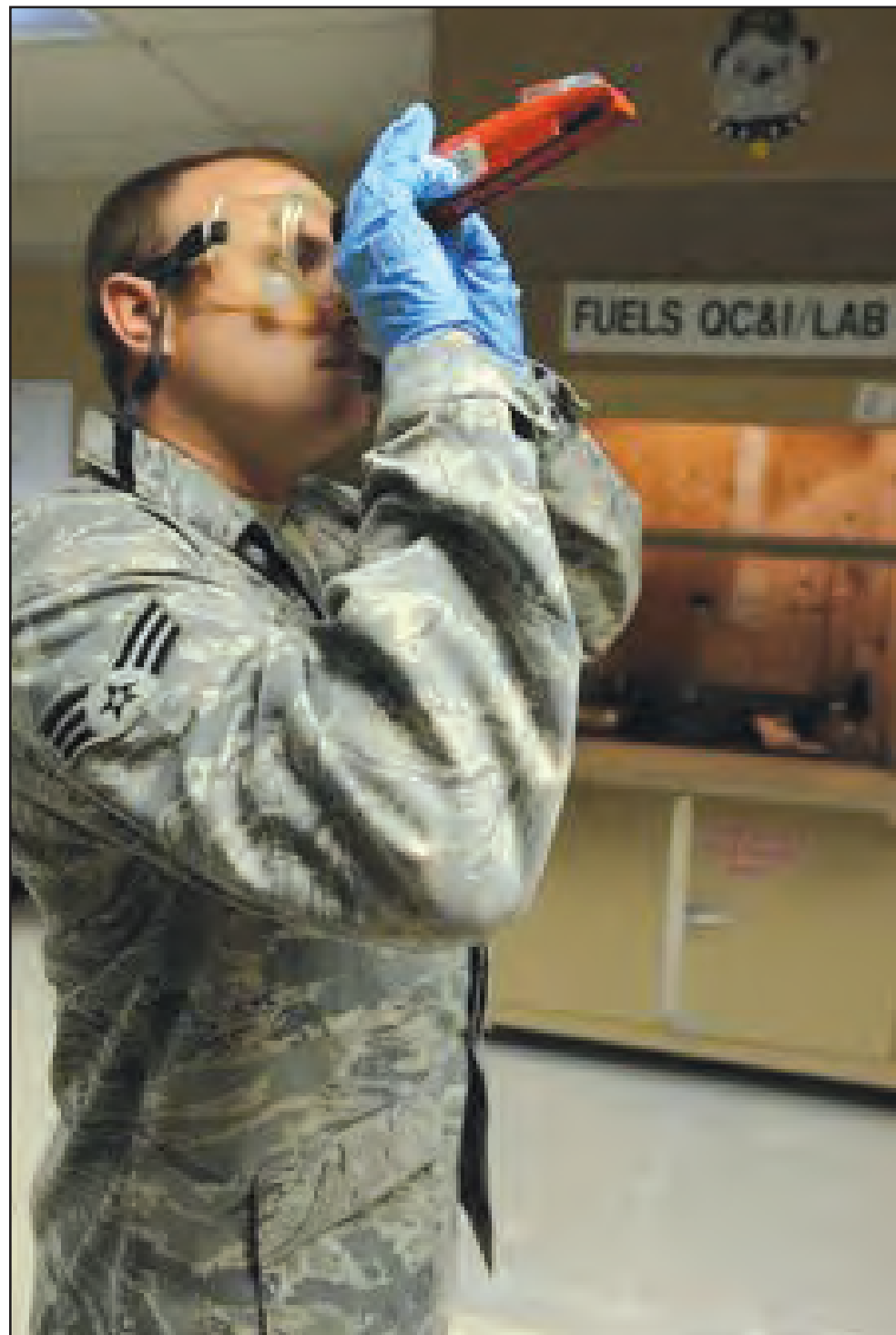
Senior Airman Matthew Dickman, 509th Logistics Readiness Squadron fuels lab tests the fizz in the fuel which will show the water content in the fuel, Aug. 11.
