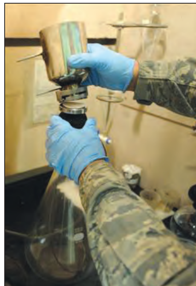
Senior Airman Matthew Dickman, 509th Logistics Readiness Squadron fuels lab, attaches the filter to the top of the large beaker, Aug. 11.
