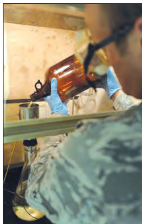
Senior Airman Matthew Dickman, 509th Logistics Readiness Squadron fuels lab tests the fizz in the fuel which will show the water content in the fuel, Aug. 11.
